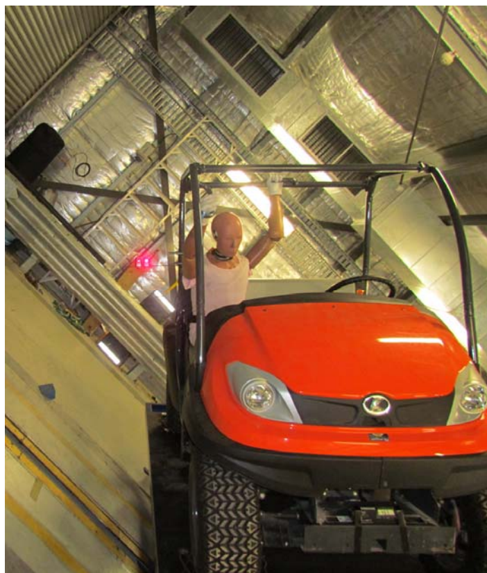
Side by Side Vehicle occupant retention – Test GI40056
