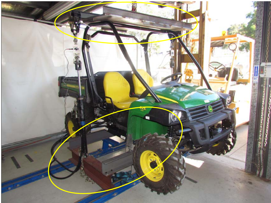
Roll Over Protective Structure vertical test steel frame (under vehicle) and load plate (on top of ROPS)
