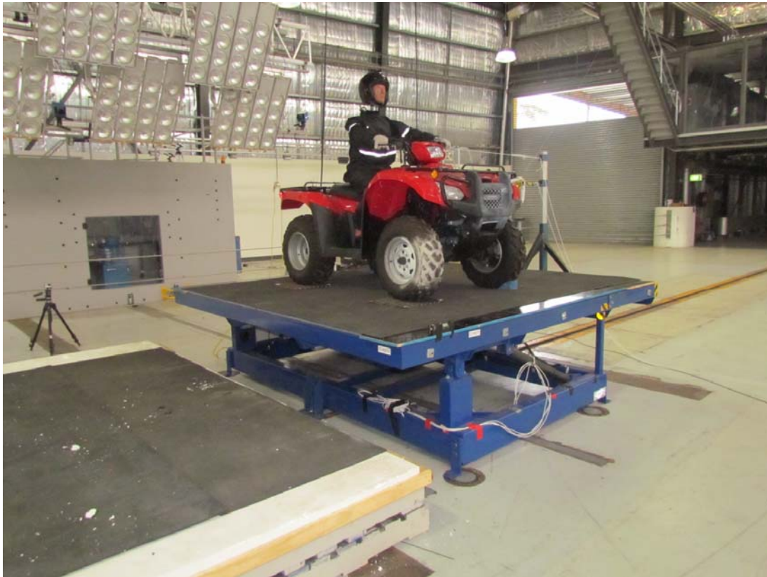
Vehicle and occupant rollover – typical test setup, quadbike lateral roll
