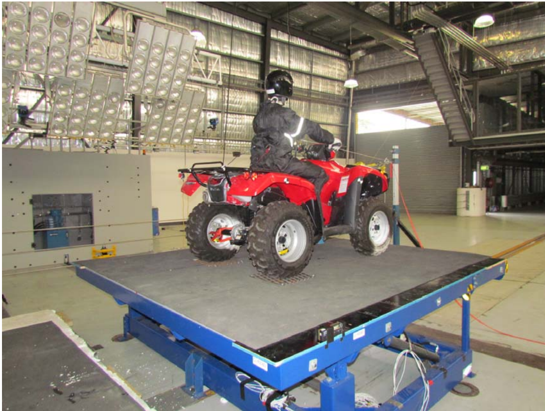
Vehicle and occupant rollover – typical test setup, quadbike rearward pitch
