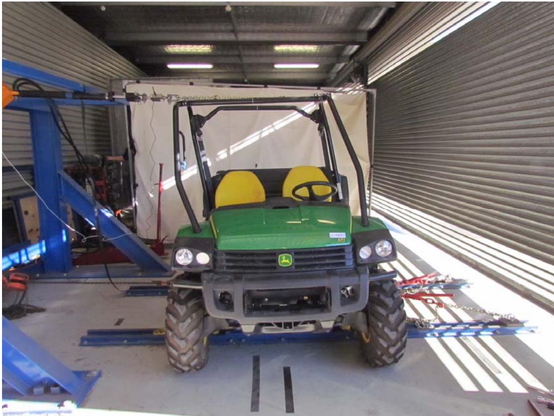
SSV ROPS test – Lateral test GI40093
