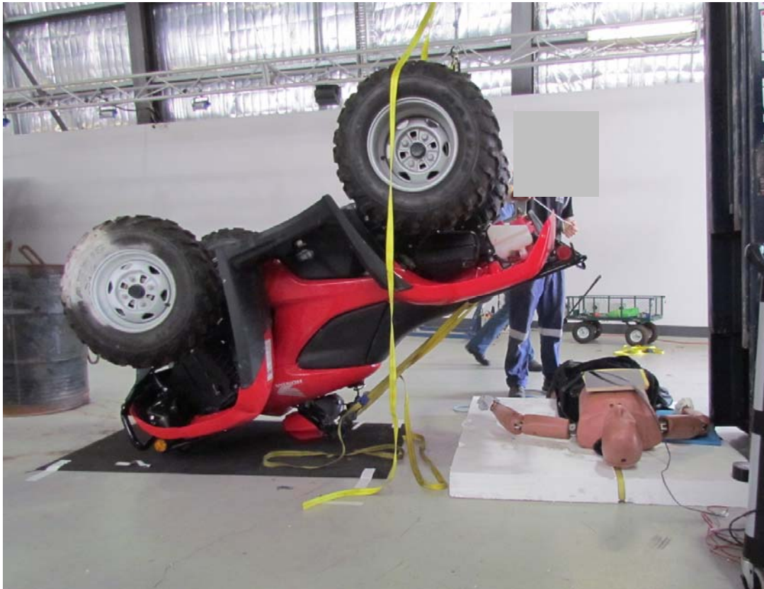
MATD chest compression – test setup, 500mm drop of quadbike rear tray onto MATD sternum
