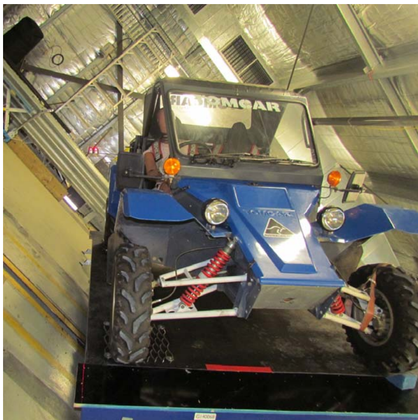
Side by Side Vehicle occupant retention – Test GI40068
