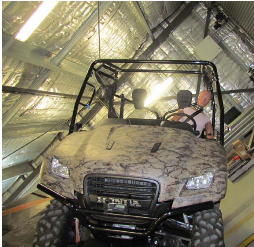
Side by Side Vehicle occupant retention – Test GI40055
