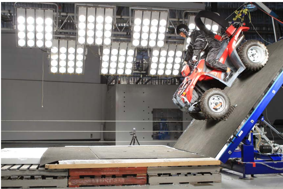
Vehicle and occupant rollover – typical test setup, quadbike forward pitch, immediately prior to vehicle and ATD release
