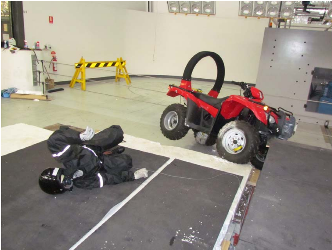
Vehicle and occupant rollover – Test GI40082 forward pitch, Lifeguard CPD, vehicle rest position
