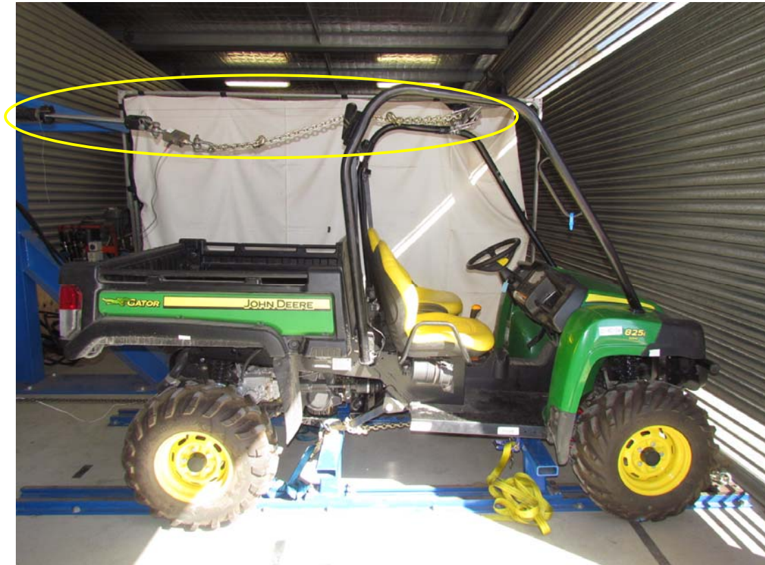
ROPS test – Longitudinal pull typical setup. Vehicle secured to mounting stands. Hydraulic cylinder, load cell & chain secured between Rigid test fixture and vehicle ROPS
