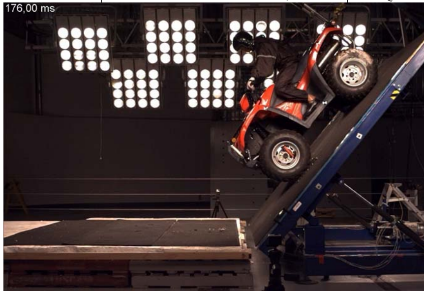
Vehicle and occupant rollover – Test G140085, forward pitch Quadbar
