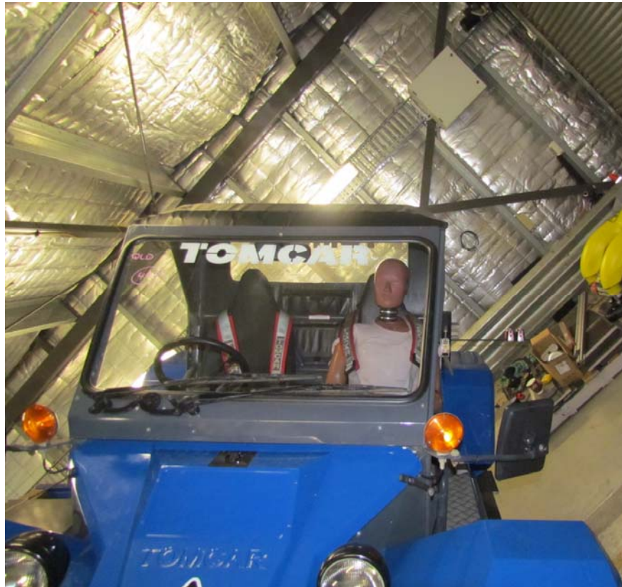
Side by Side Vehicle occupant retention – Test GI40067
