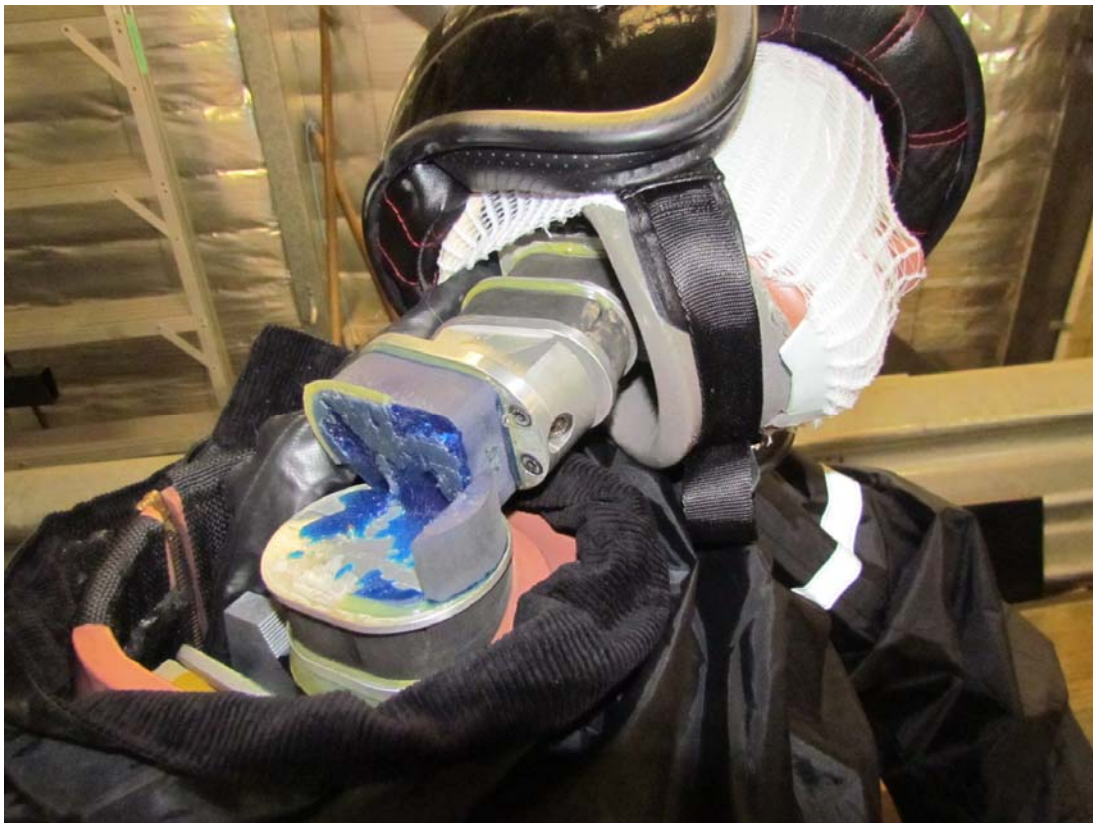
Vehicle and occupant rollover – Test latroll_00, damage to MATD neck
