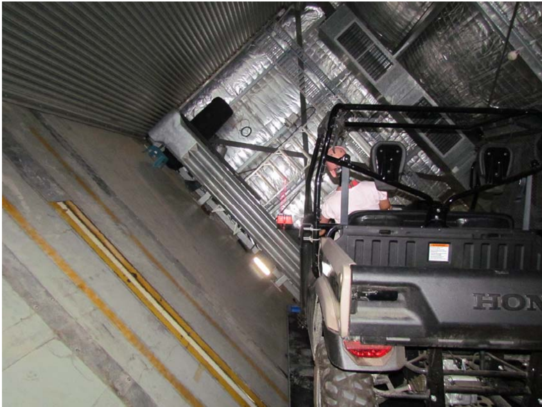
Side by Side Vehicle occupant retention – typical vehicle at 45° tilt angle with longitudinal/vertical planes projected along side vehicle located 127mm and 178mm from widest point of vehicle
