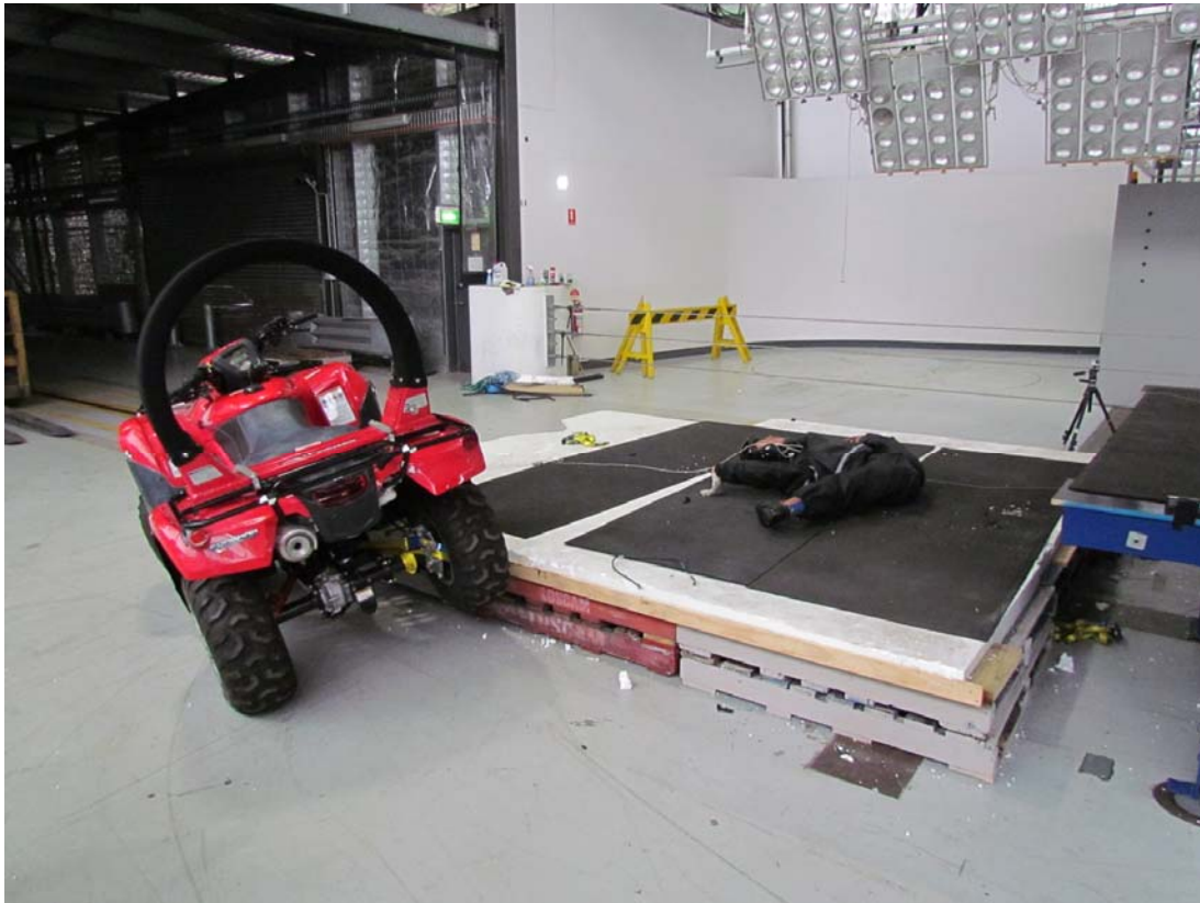
Vehicle and occupant rollover – Test G140079 rearward pitch, Lifeguard CPD, vehicle rest position
