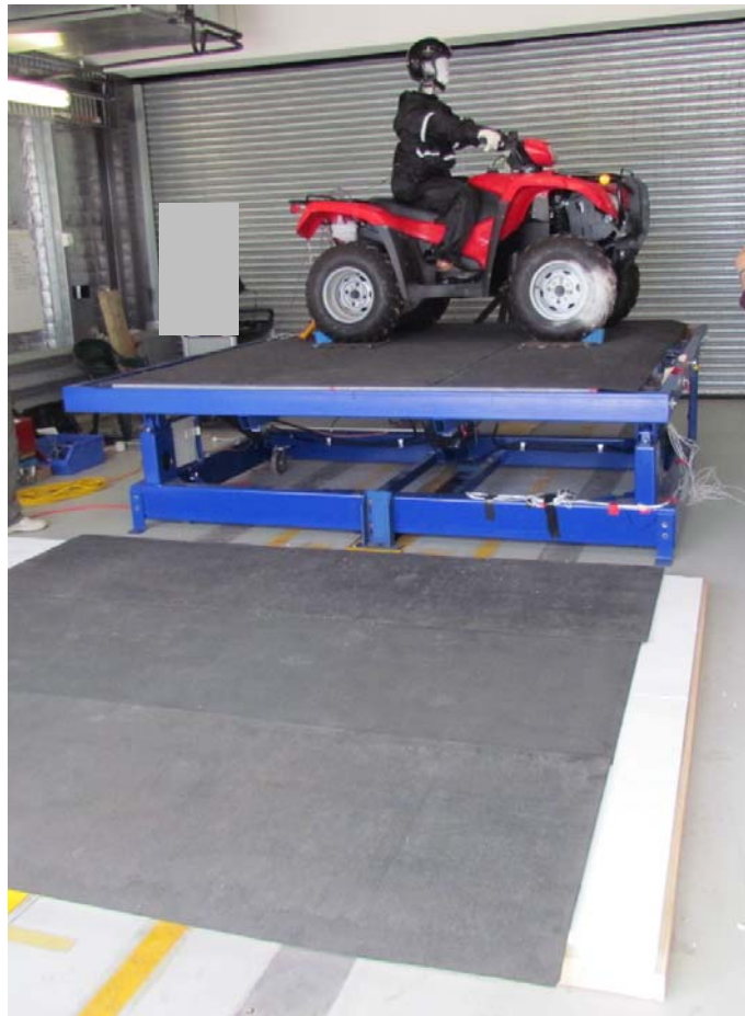
Vehicle and occupant rollover – test setup latroll_00
