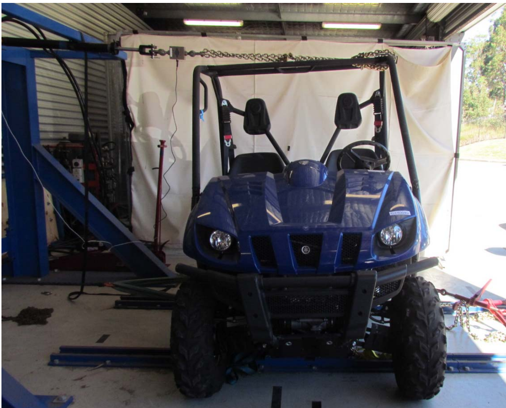
SSV ROPS test – Lateral test GI40092
