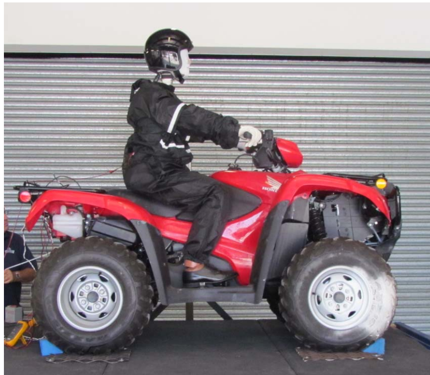
Vehicle and occupant rollover – test setup latroll_00
