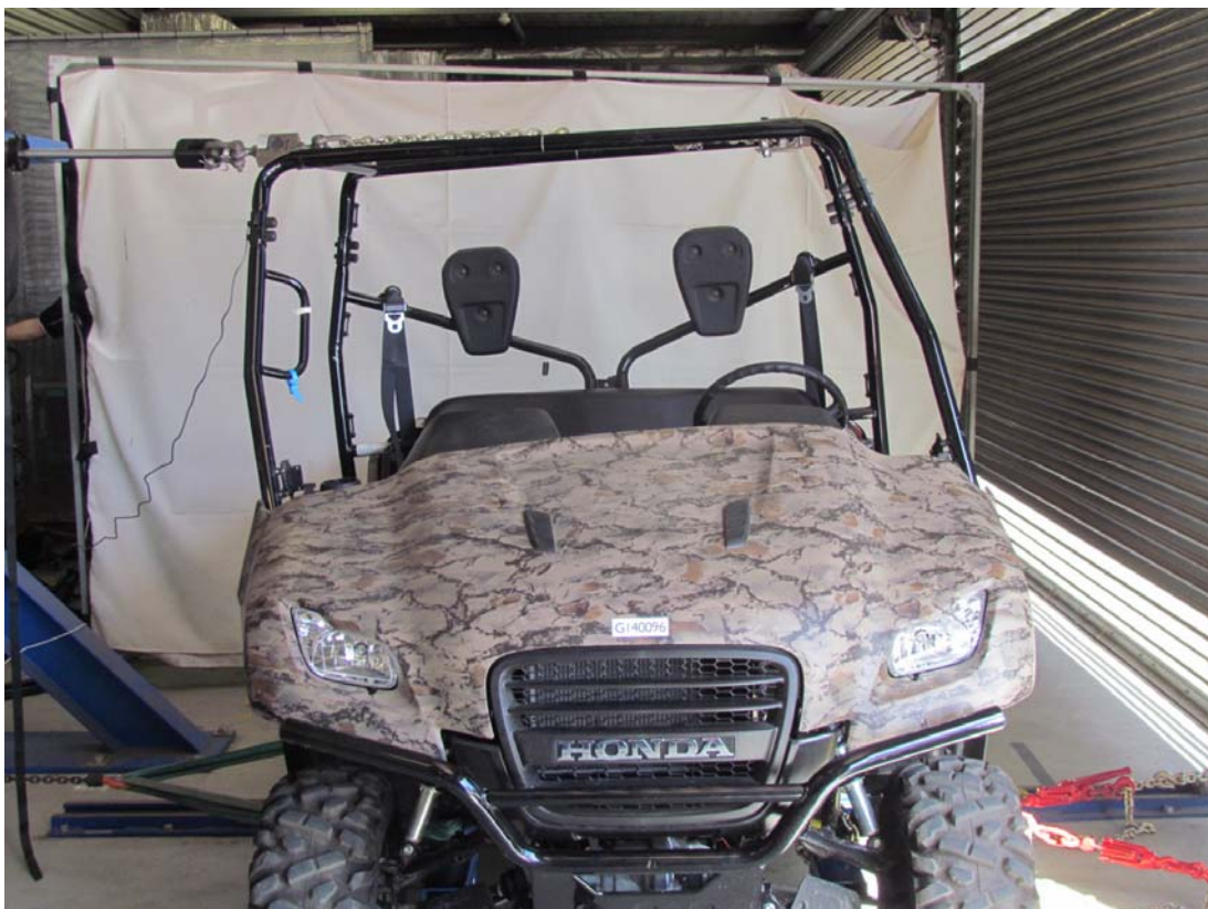
SSV ROPS test – Lateral test GI40096
