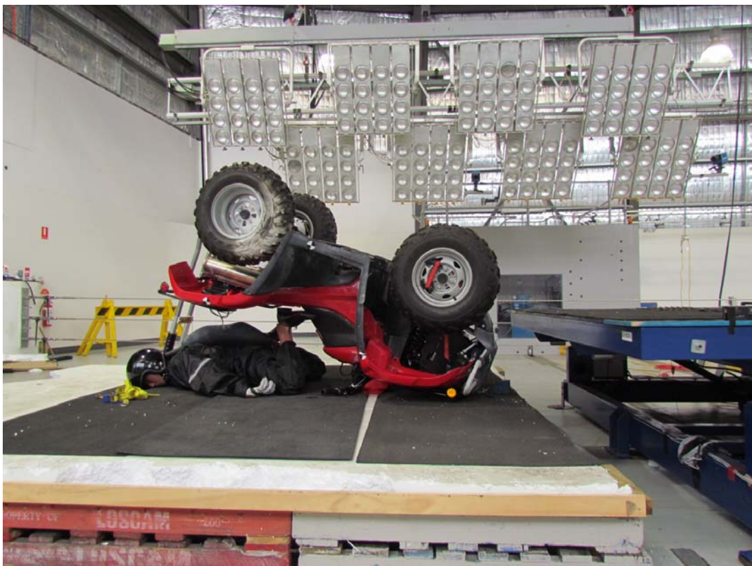
Vehicle and occupant rollover – Test GI40085 forward pitch, Quadbar CPD, vehicle rest position
