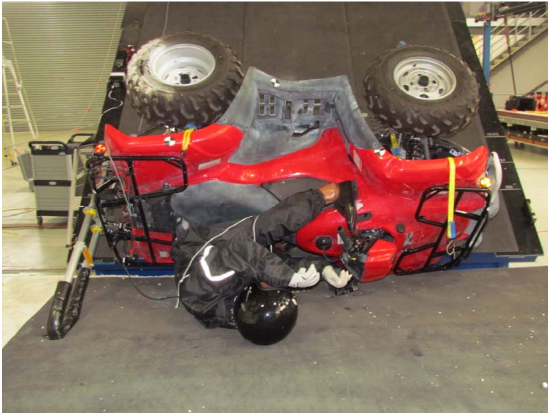
Vehicle and occupant rollover – Test G140077 lateral roll, Quadbar CPD, vehicle rest position
