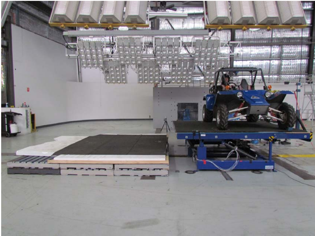
Vehicle and occupant rollover – typical test setup, SSV lateral roll
