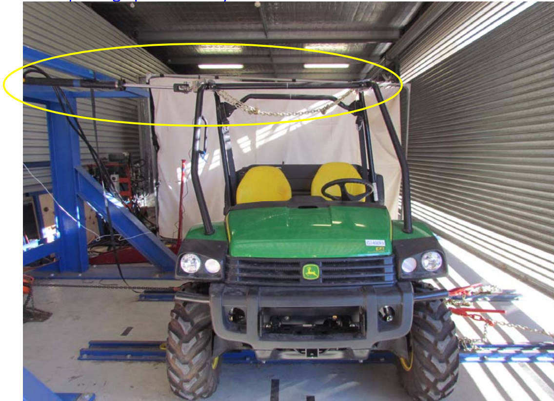
ROPS test – Lateral pull typical setup. Vehicle secured to mounting stands. Hydraulic cylinder, load cell & chain secured between Rigid test fixture and vehicle ROPS
