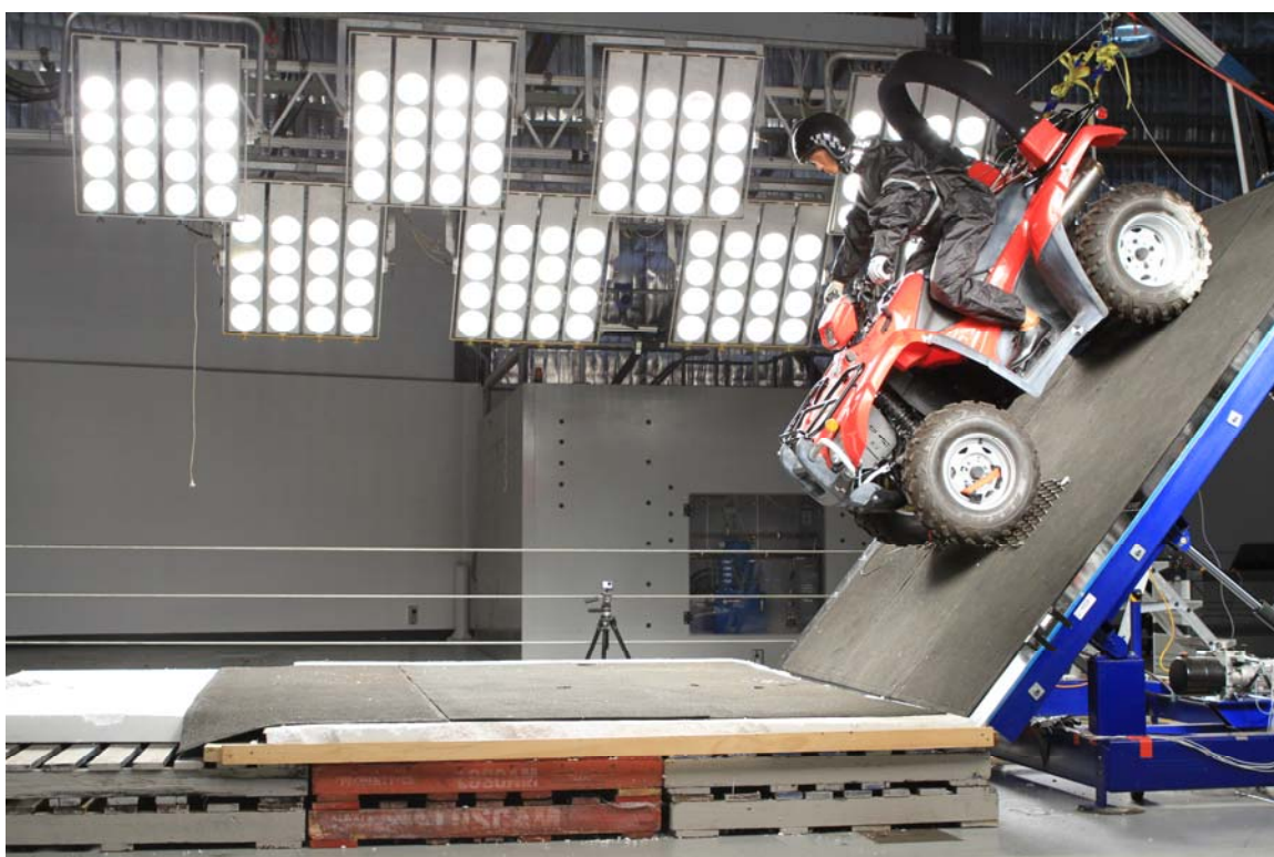
Figure 4 – Rollover test with occupant, test in progress
