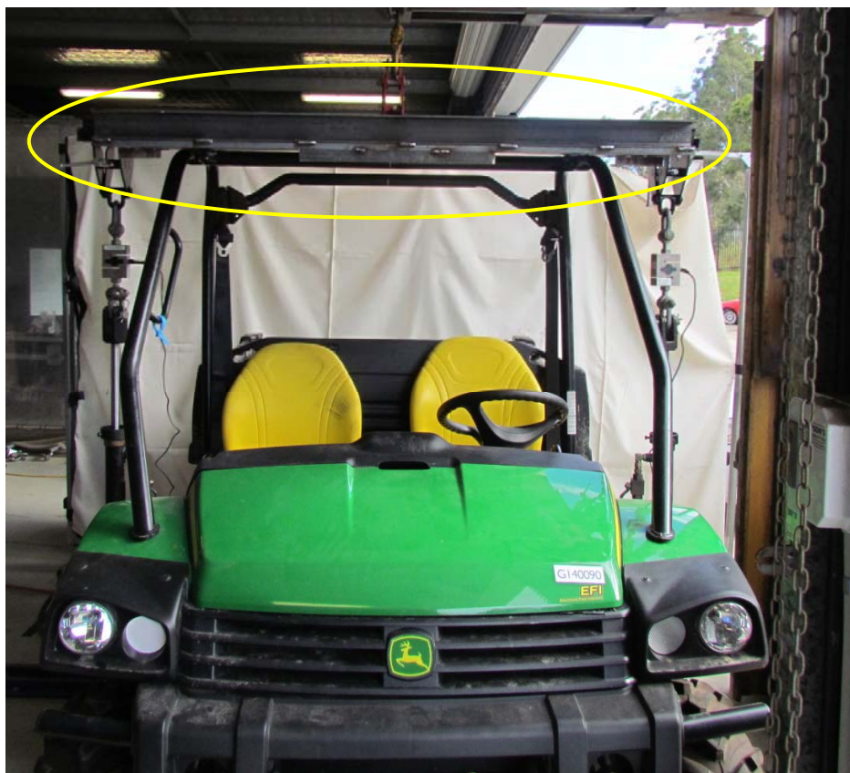
ROPS test – Vertical pull typical setup. Rigid top plate aligned with ROPS centreline
