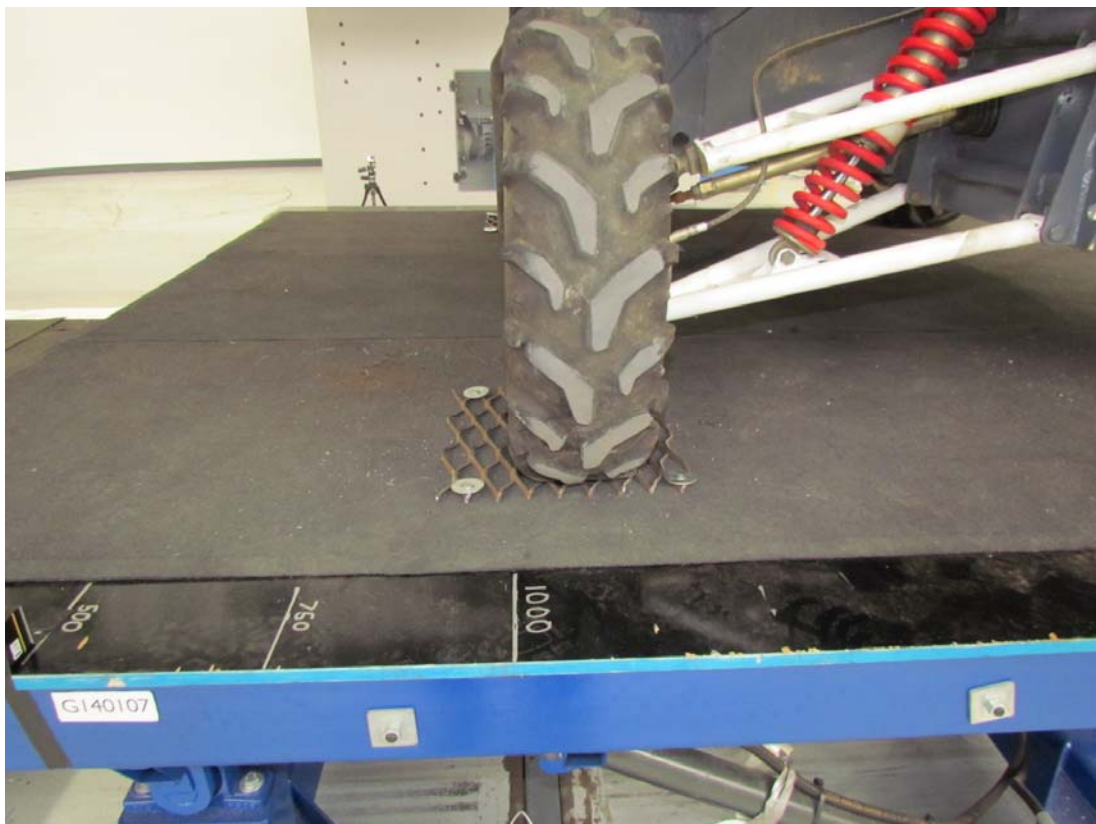
Tilt table top surface with expanded mesh anti-slip plates located under vehicle tyres
