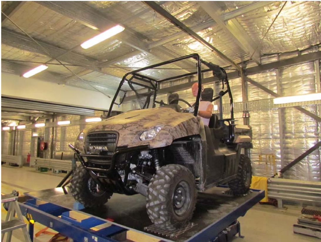
Side by Side Vehicle occupant retention – typical vehicle setup on tilt table
