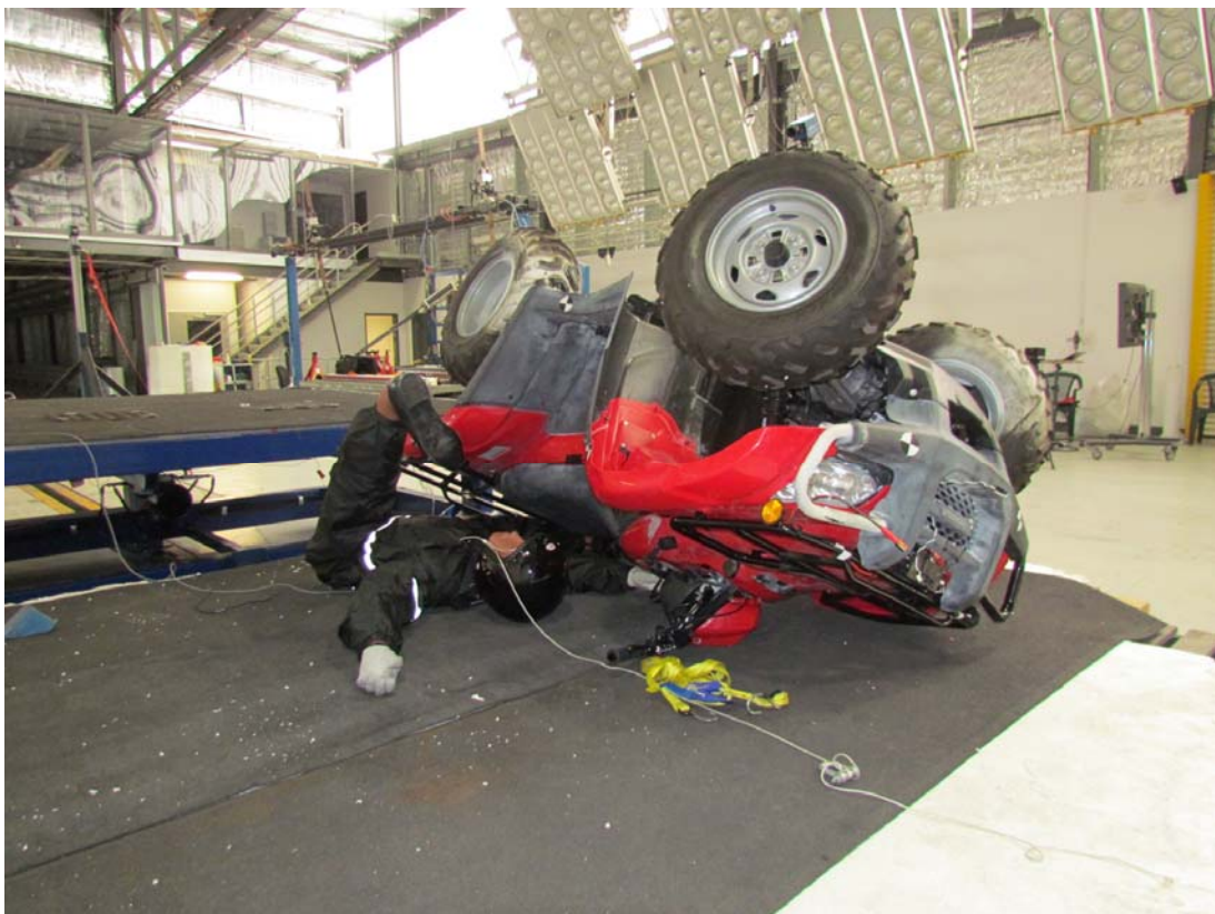
Vehicle and occupant rollover – Test G140080 rearward pitch, No CPD, vehicle rest position
