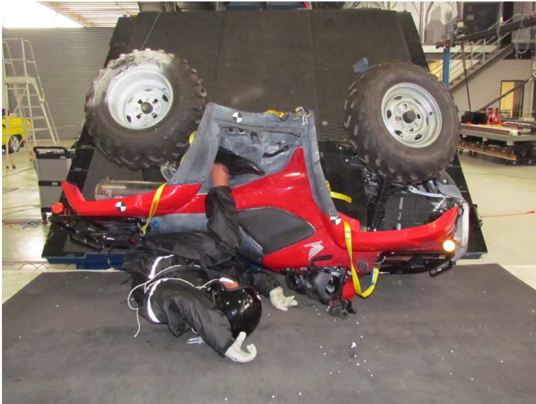
Vehicle and occupant rollover – Test GI 40075 lateral roll, No CPD, vehicle rest position
