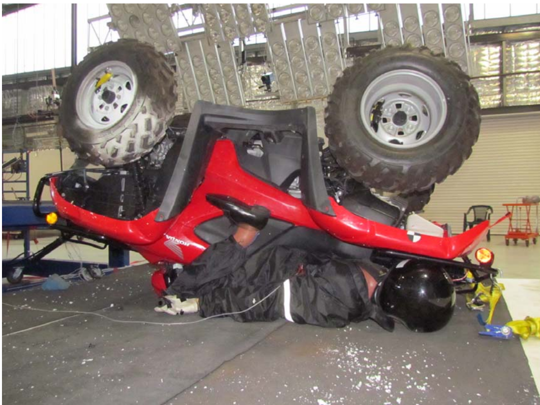
Vehicle and occupant rollover – Test GI40088 forward pitch, No CPD, vehicle rest position
