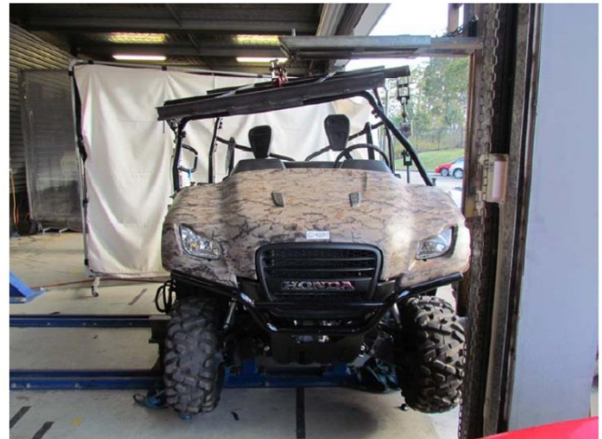
Vertical loading reaches 88% of ANSI/ROHVA 1-2011 requirements after which test was stopped.
