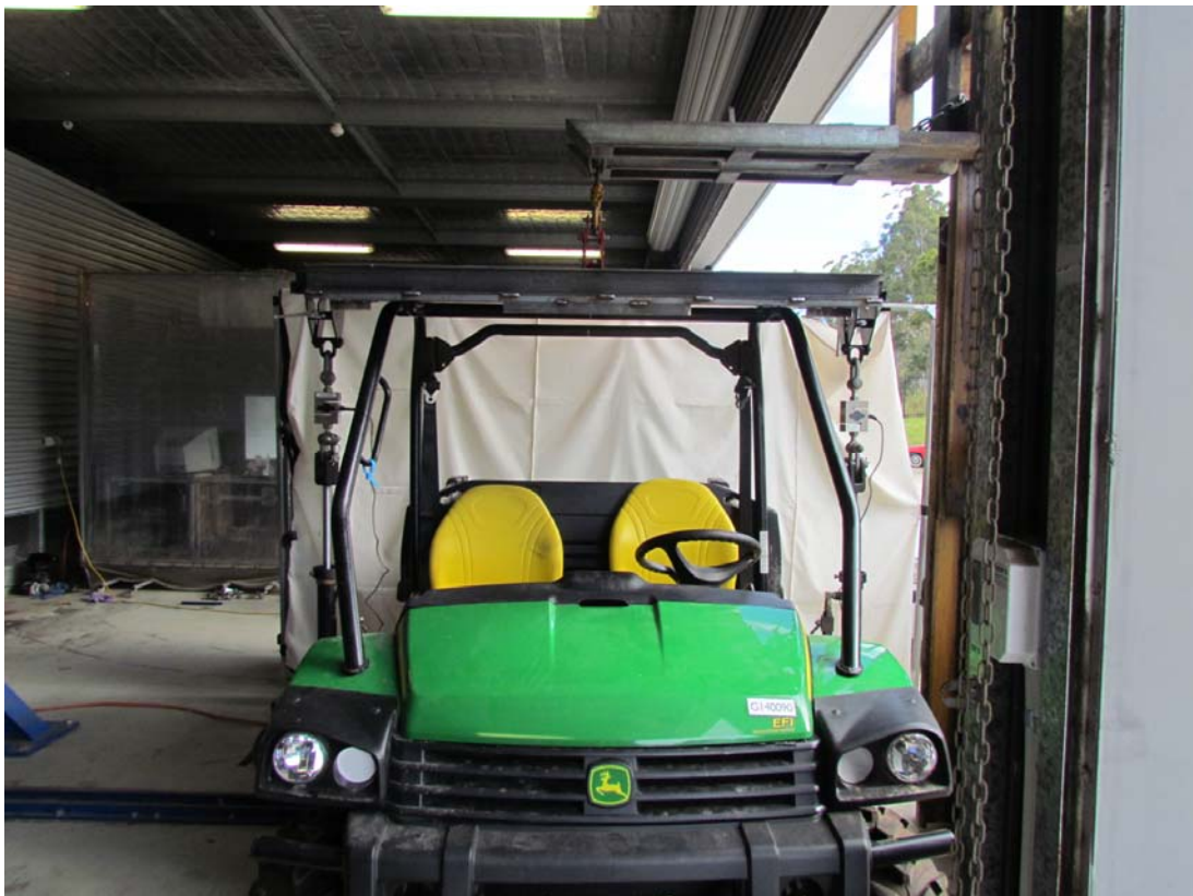
SSV ROPS test – Vertical test G140090
