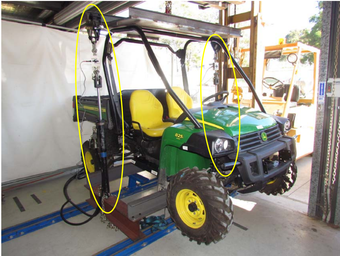
ROPS test – Vertical pull typical setup. Vehicle secured to steel frame under chassis. Two hydraulic cylinders & load cells secured between Rigid top plate and steel frame under vehicle
