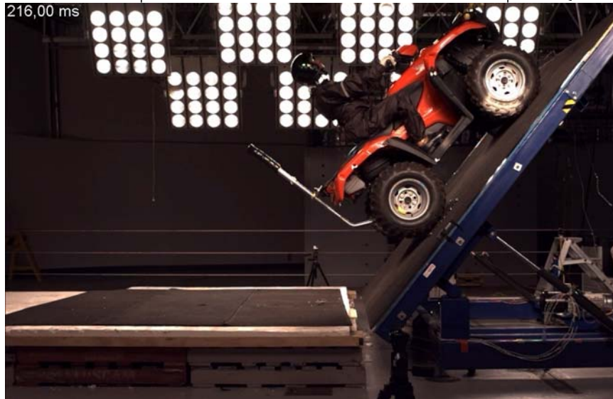
Vehicle and occupant rollover – Test G140078, rearward pitch Quadbar
