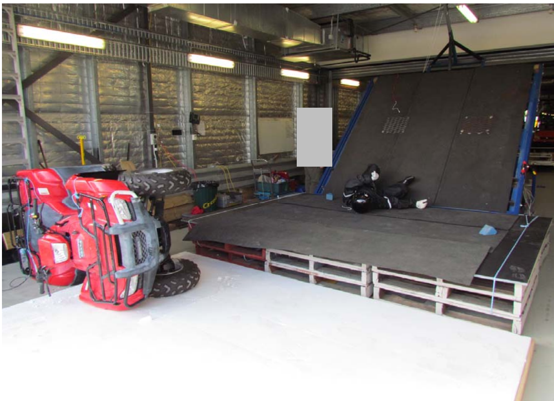
Vehicle and occupant rollover – Test latroll_01 vehicle rest position
