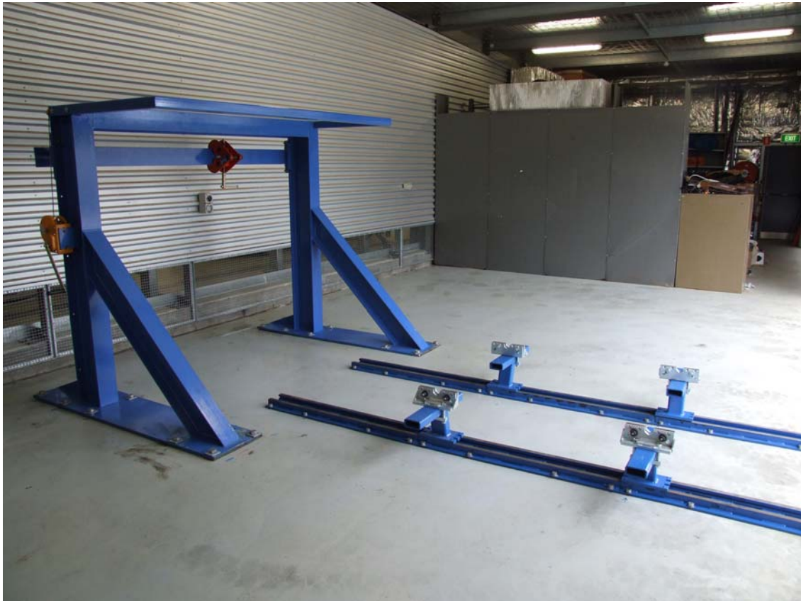
Roll-Over Protective Structure rigid steel test fixture, rails and adjustable vehicle mounting stands (lateral and longitudinal tests)
