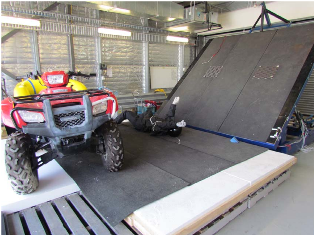
Vehicle and occupant rollover – Test latroll_02 vehicle rest position
