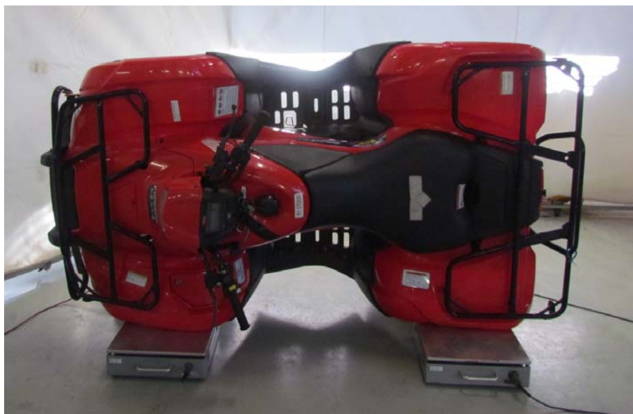
Figure 1 – Quad bike ground contact force test in progress
