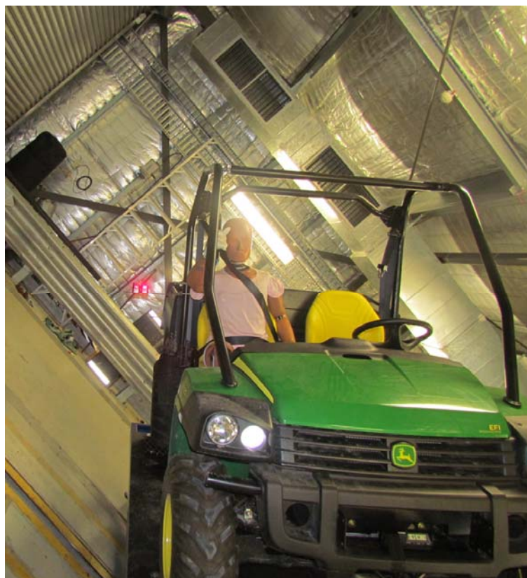
Side by Side Vehicle occupant retention – Test GI40060
