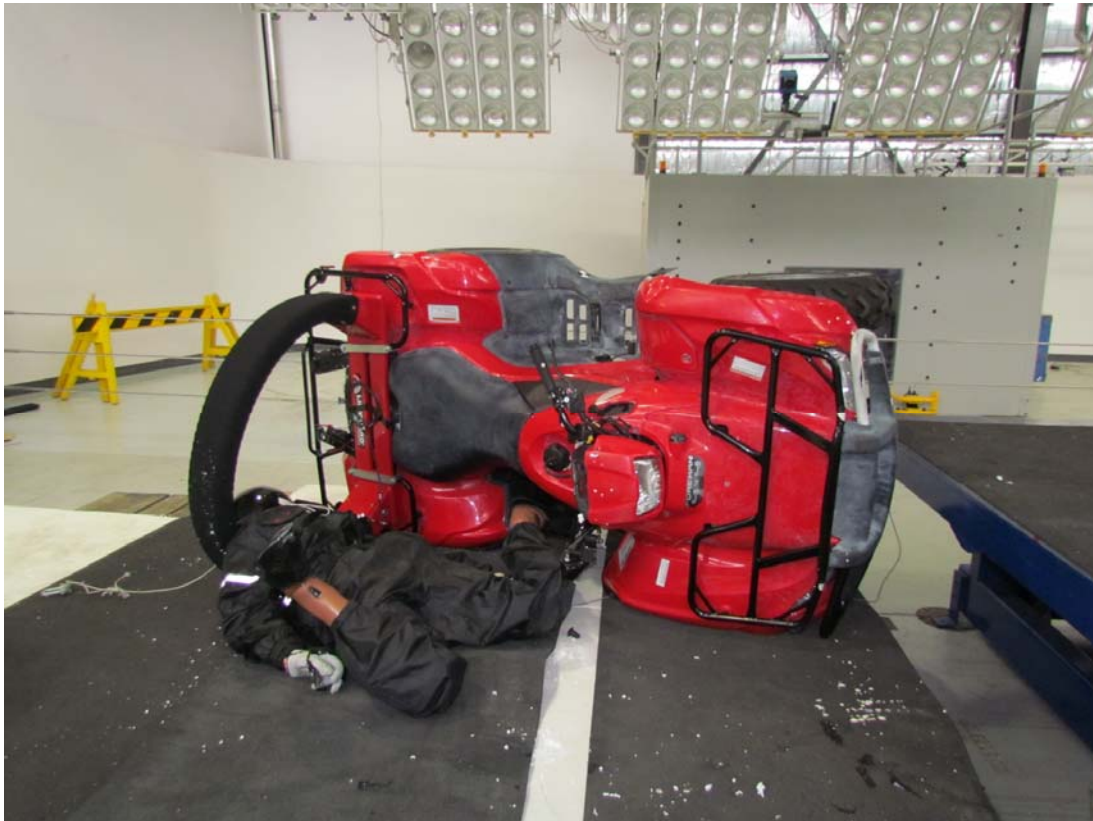
Vehicle and occupant rollover – Test GI40087 forward pitch, Lifeguard CPD, vehicle rest position
