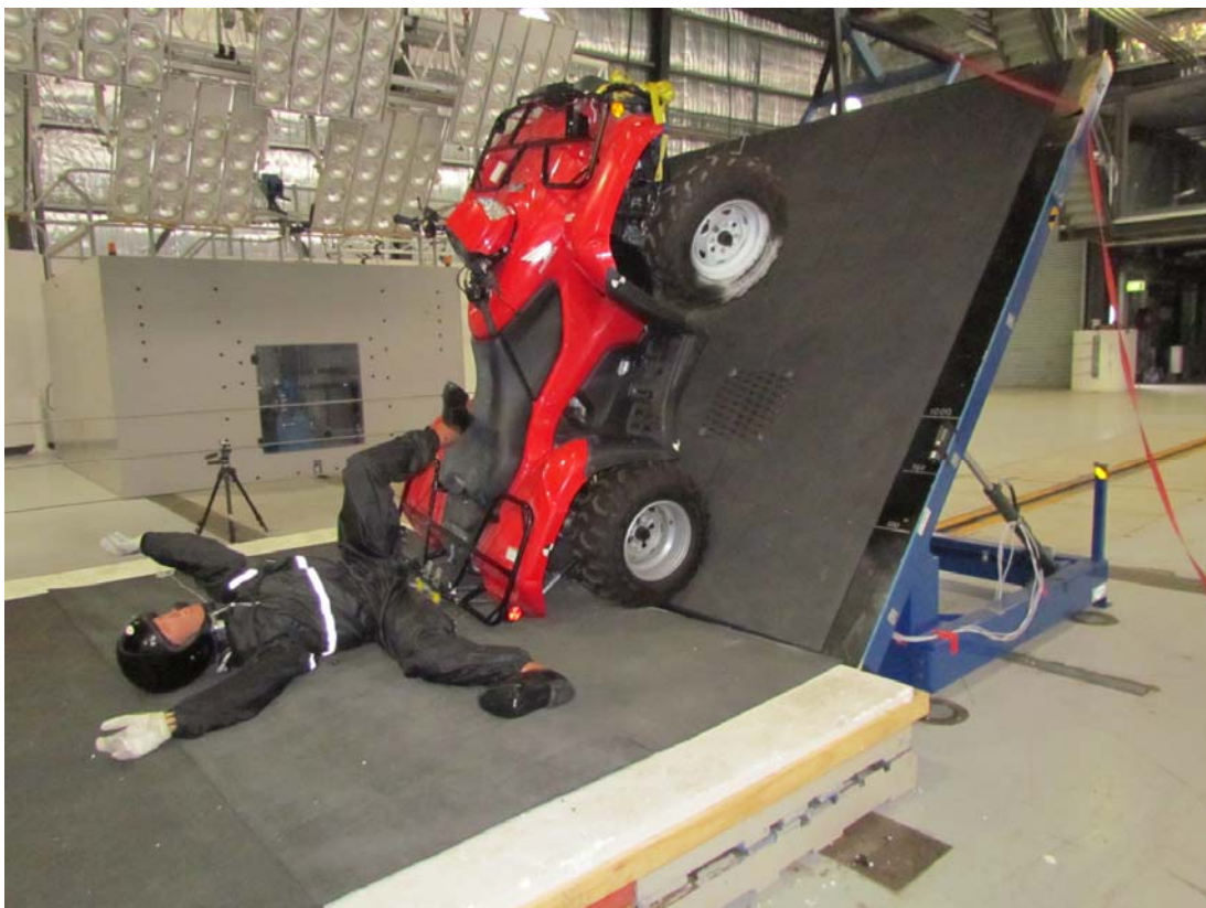
Vehicle and occupant rollover – Test G140078 rearward pitch, Quadbar CPD, vehicle rest position
