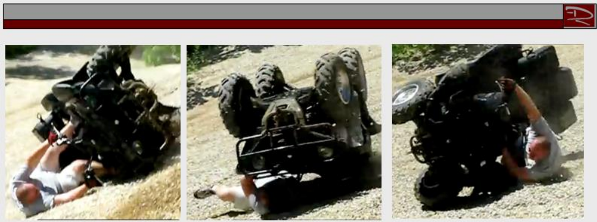
Figure 3: Van Ee et al. (2012) demonstrate how a Quad bike can roll laterally over a rider without causing any injury. The rider stood up and walked away from the incident.
