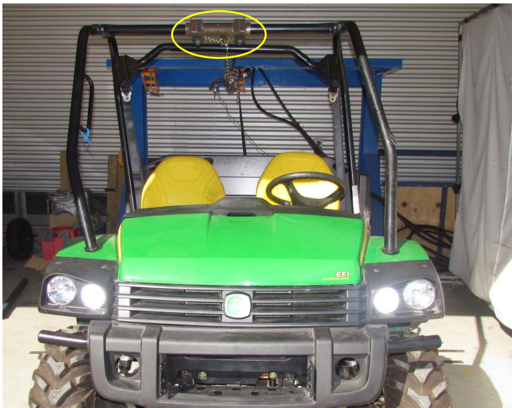
ROPS test – Lateral pull typical setup, Load Distribution Device (LDD) aligned with ROPS centreline
