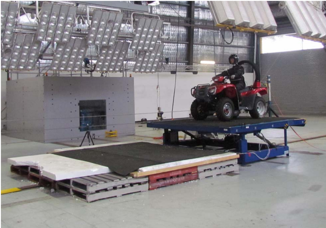
Vehicle and occupant rollover – typical test setup, quadbike forward pitch
