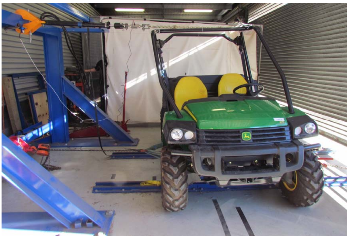
Figure 3 – SSV Roll-Over Protective Structure (ROPS) lateral pull test in progress
