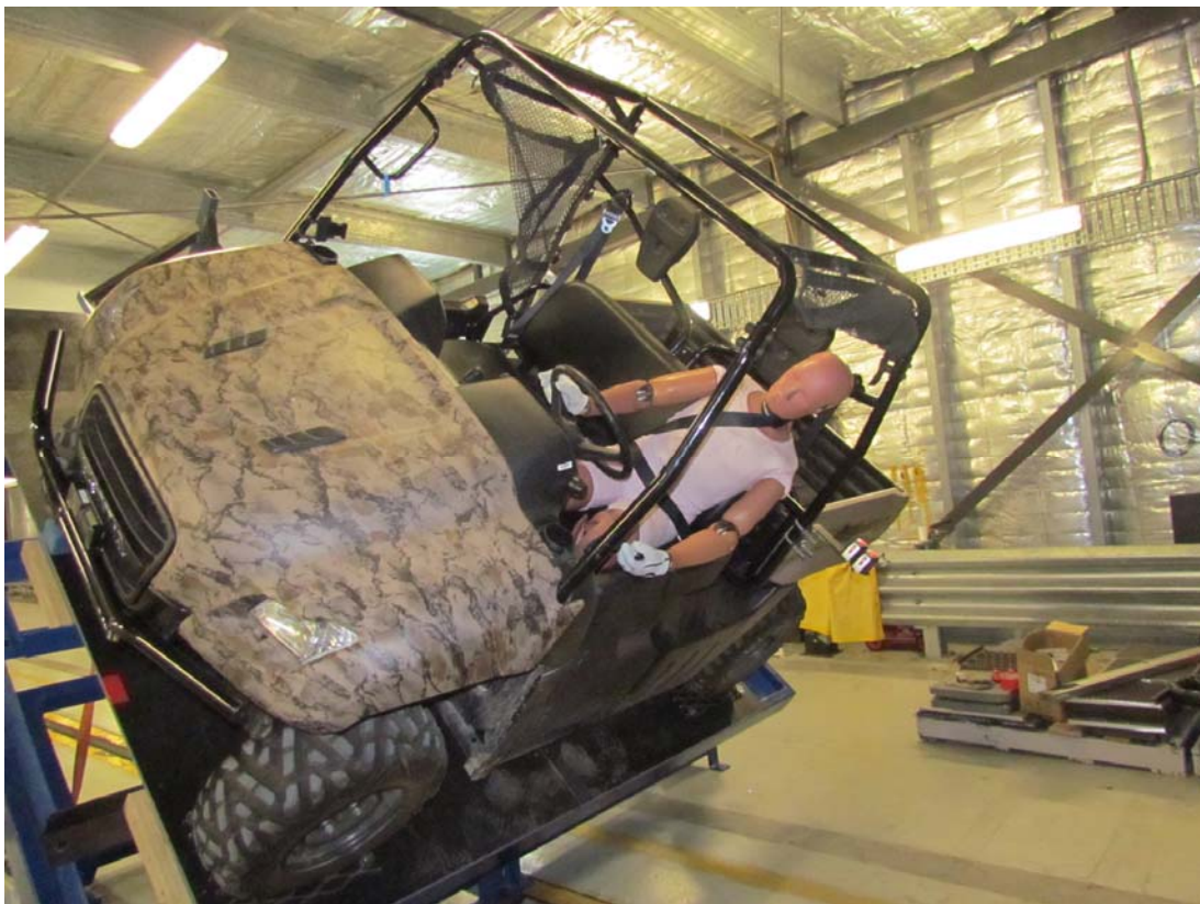
Side by Side Vehicle occupant retention – typical vehicle at 45° tilt angle
