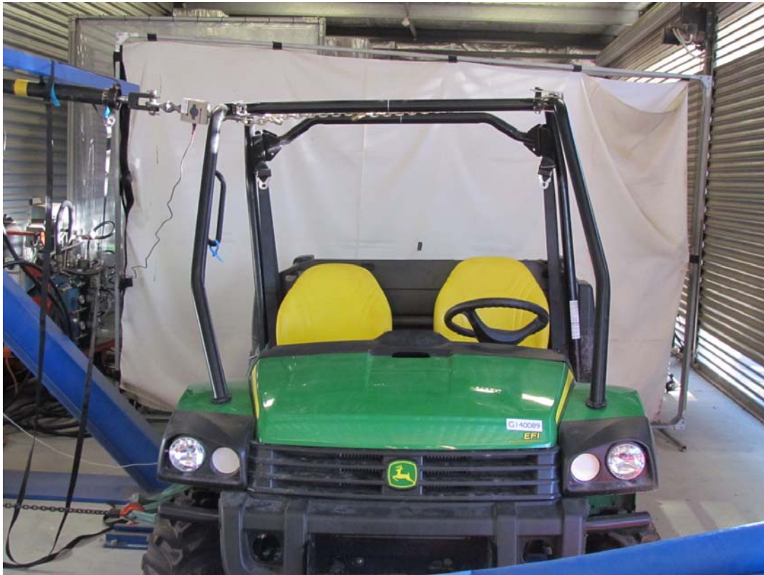
SSV ROPS test – Lateral test G140089
