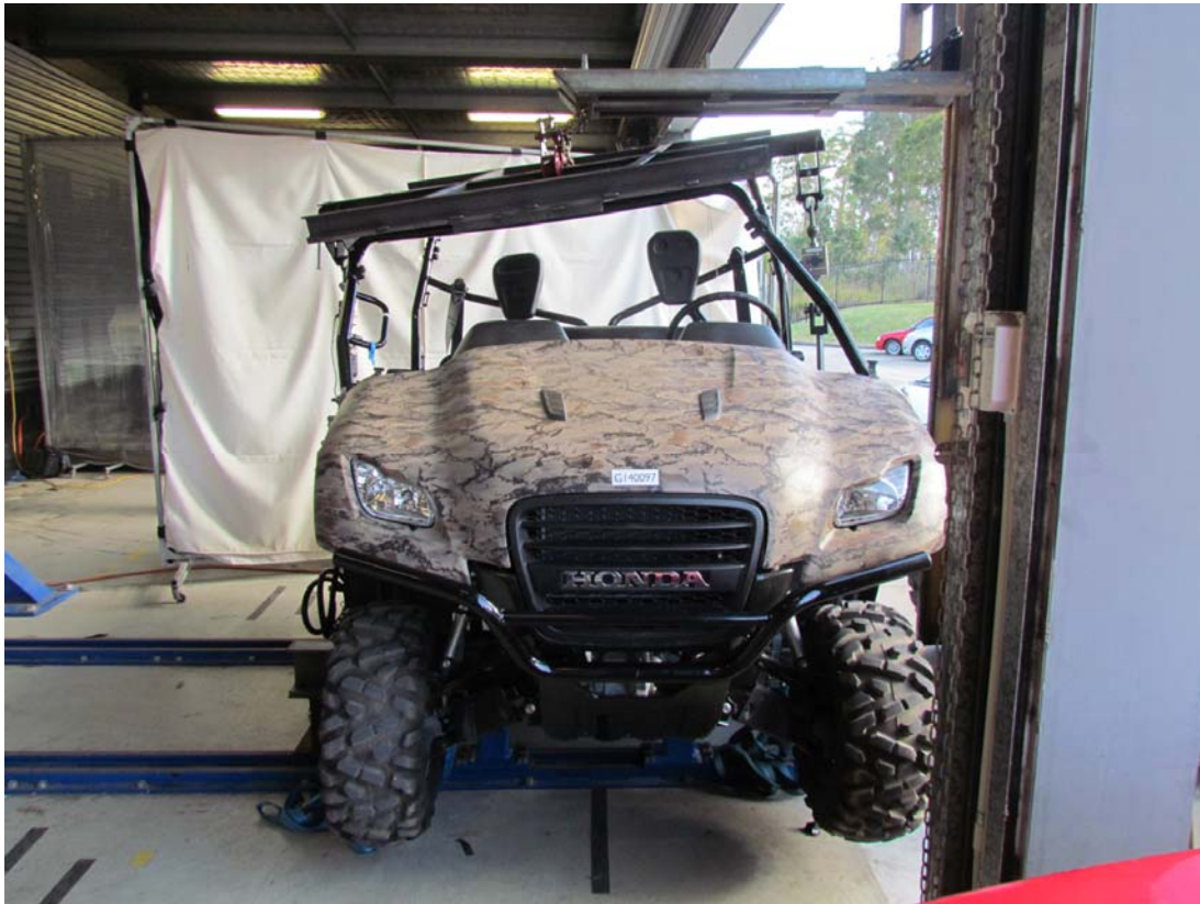
SSV ROPS test – Vertical test GI40097
