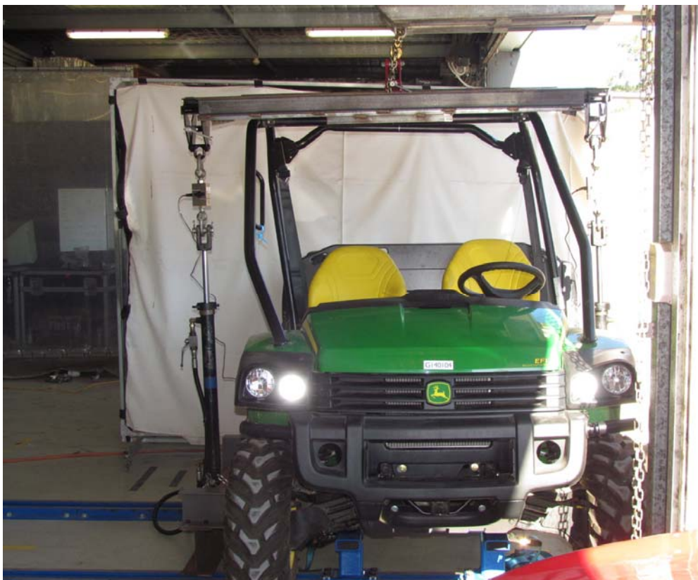
SSV ROPS test – Vertical test GI40104
