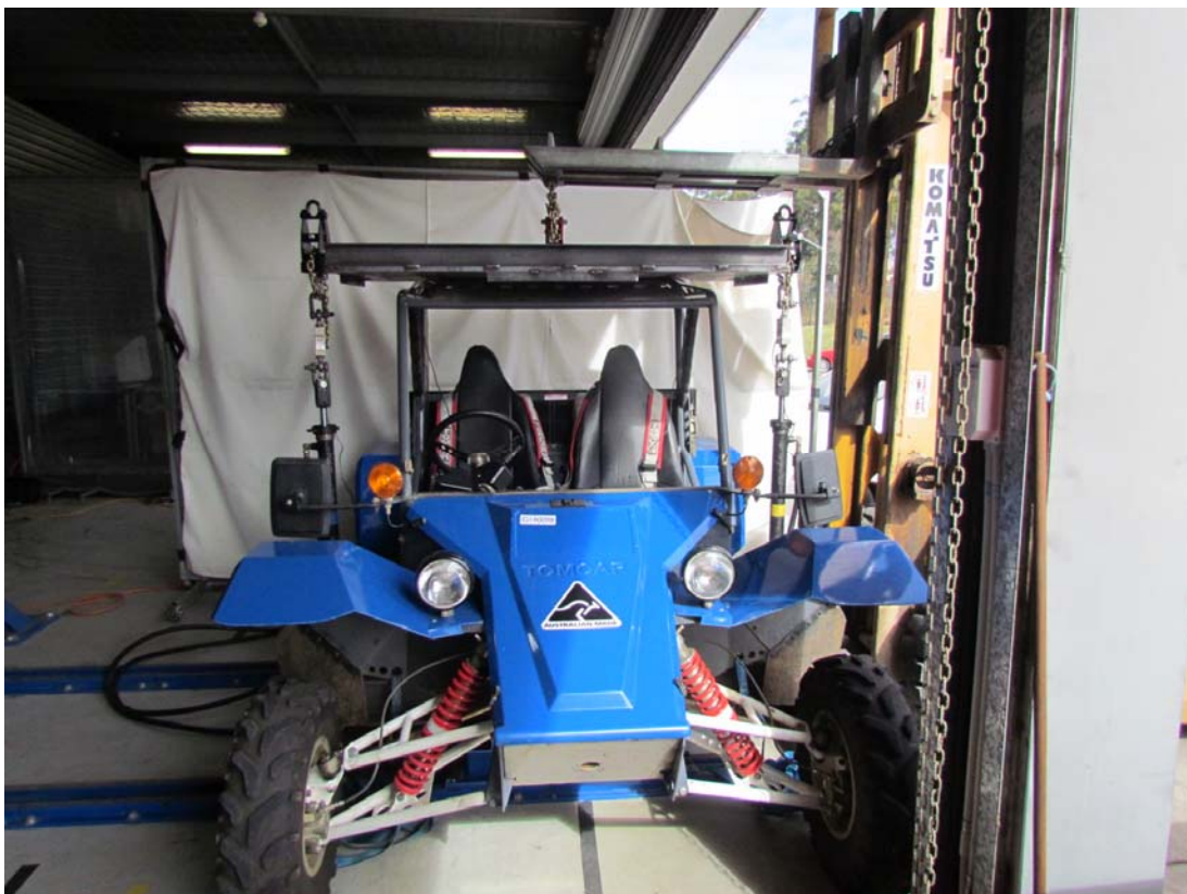
SSV ROPS test – Vertical test GI40098
