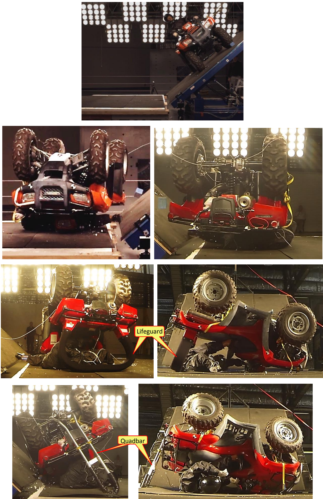
Figure 8: Quad Tests: Lateral rollover: Top – setup; 2 nd row – baseline; 3 rd row – Lifeguard OPDS; 4 th row – Quadbar OPD.
