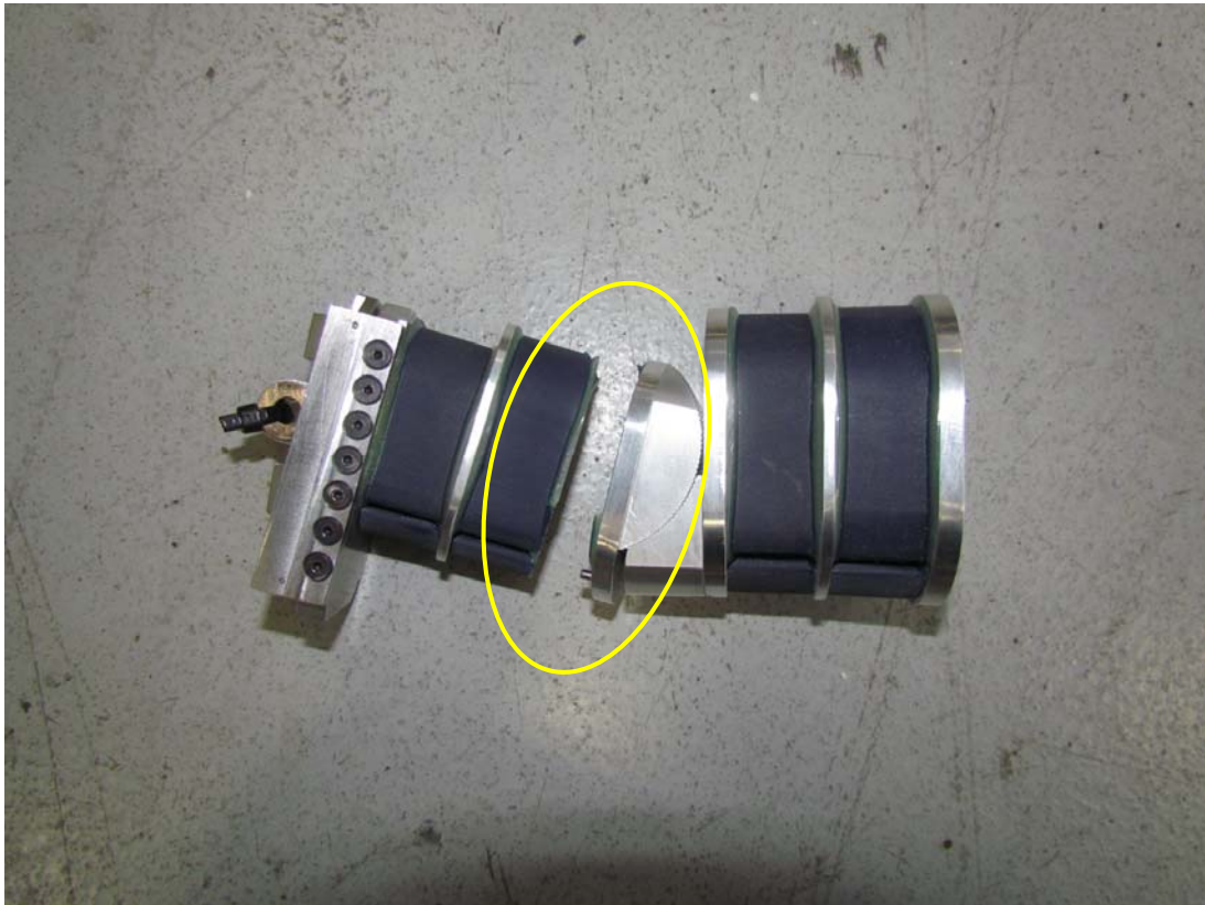
Vehicle and occupant rollover – Test GI40082, damage to MATD neck
