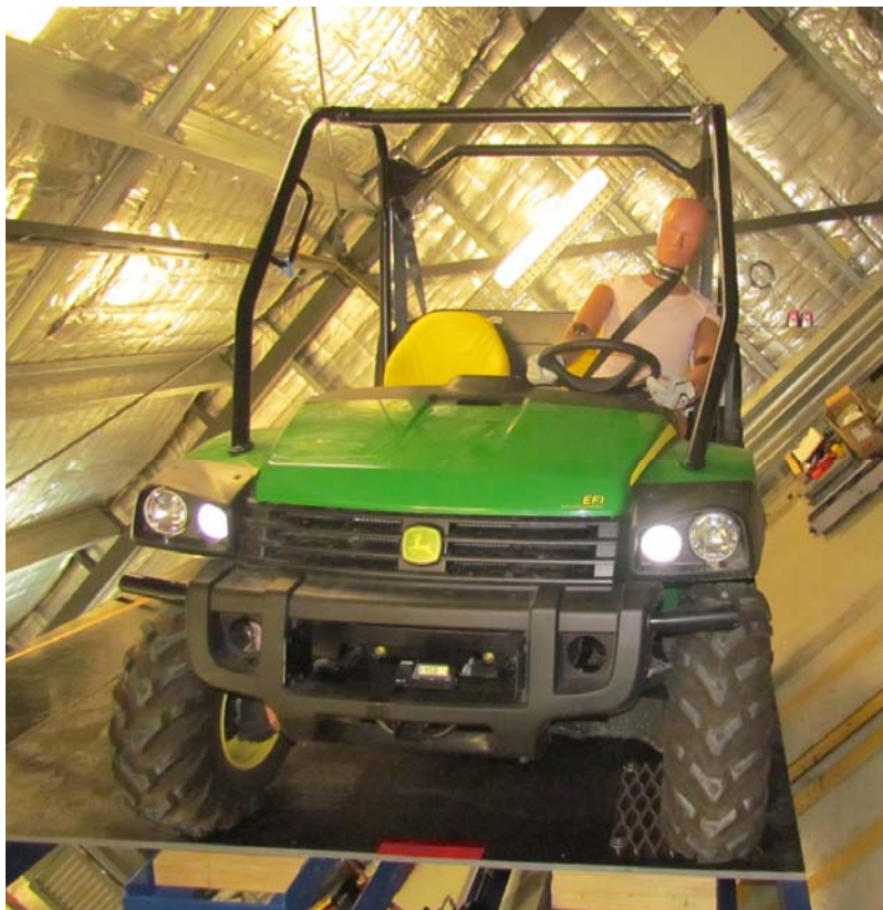
Side by Side Vehicle occupant retention – Test GI40062
