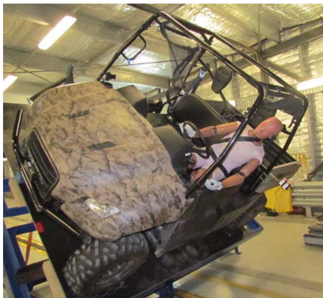
Figure 2 – Side-by-Side Vehicle occupant retention test in progress
