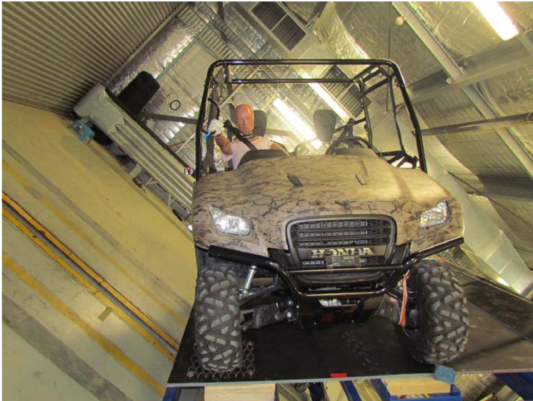
Side by Side Vehicle occupant retention – Test GI40053
