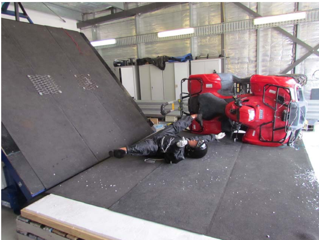
Vehicle and occupant rollover – Test rearpitch_01 vehicle rest position
