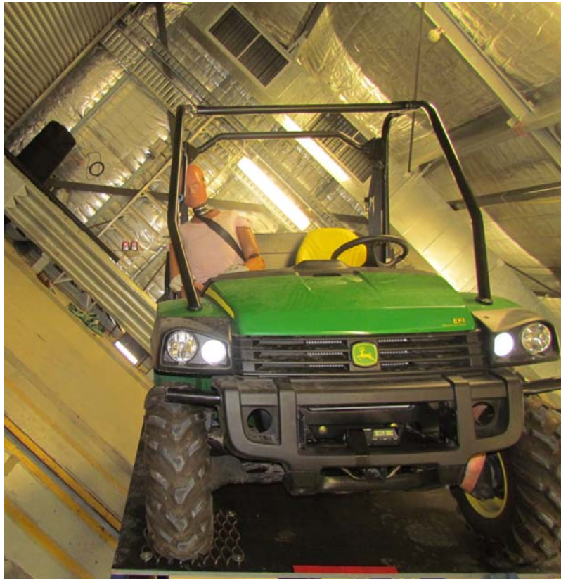
Side by Side Vehicle occupant retention – Test GI40061
