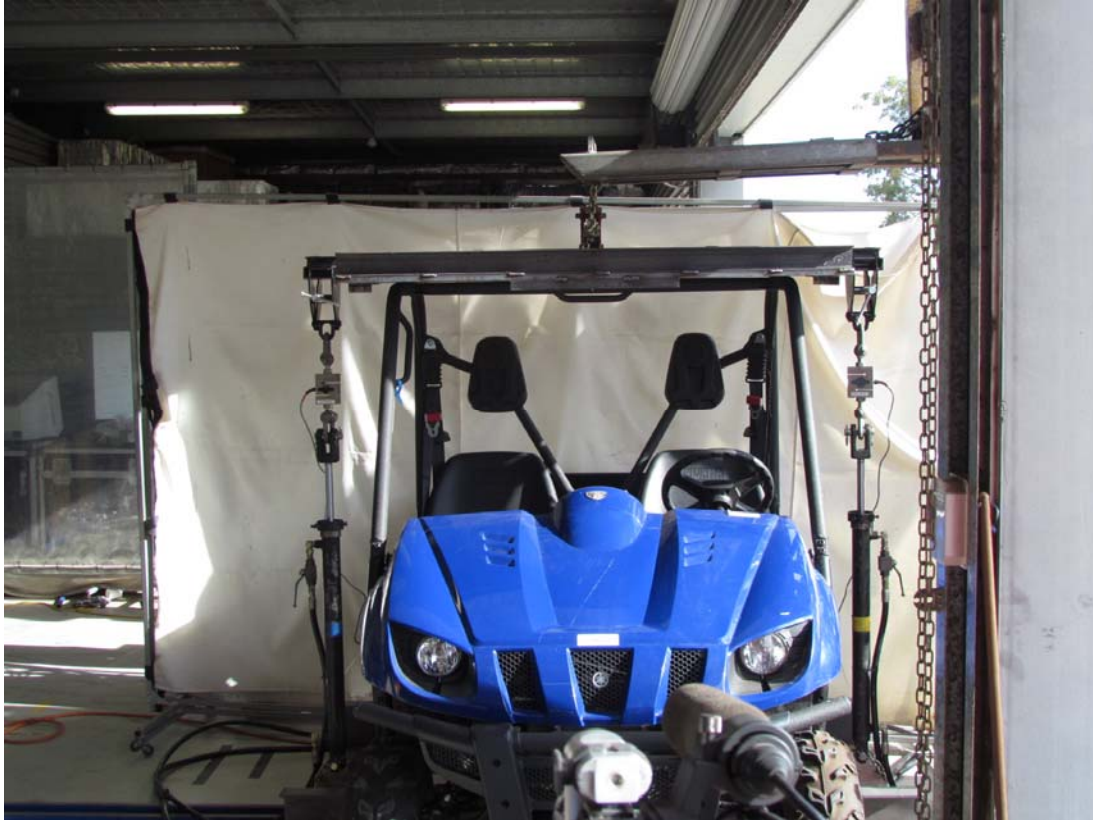
SSV ROPS test – Vertical test GI40099
