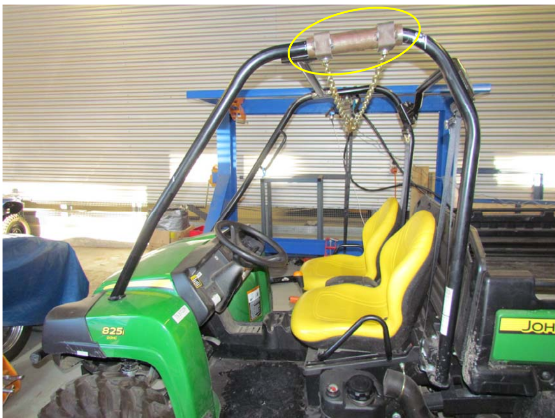
ROPS test – Lateral pull typical setup, Load Distribution Device (LDD)
