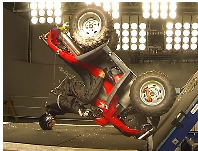
b) Forward pitch demonstrating how rider can receive serious cervical spine injury. MATD neck was fractured twice during testing.
