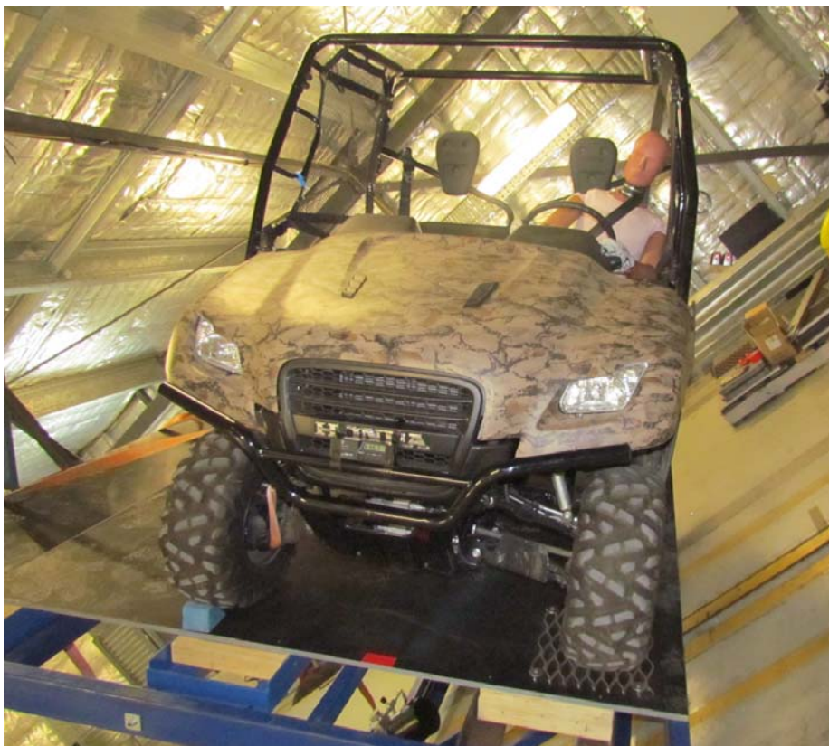
Side by Side Vehicle occupant retention – Test GI40054
