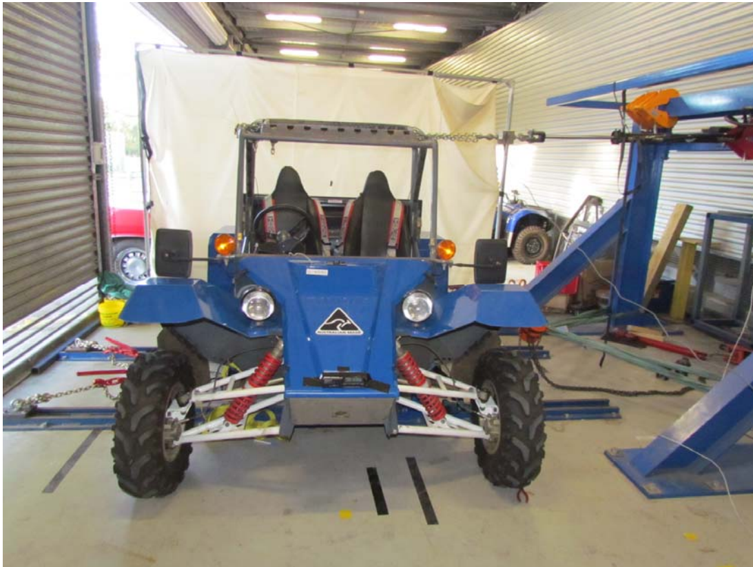
SSV ROPS test – Lateral test GI40095
