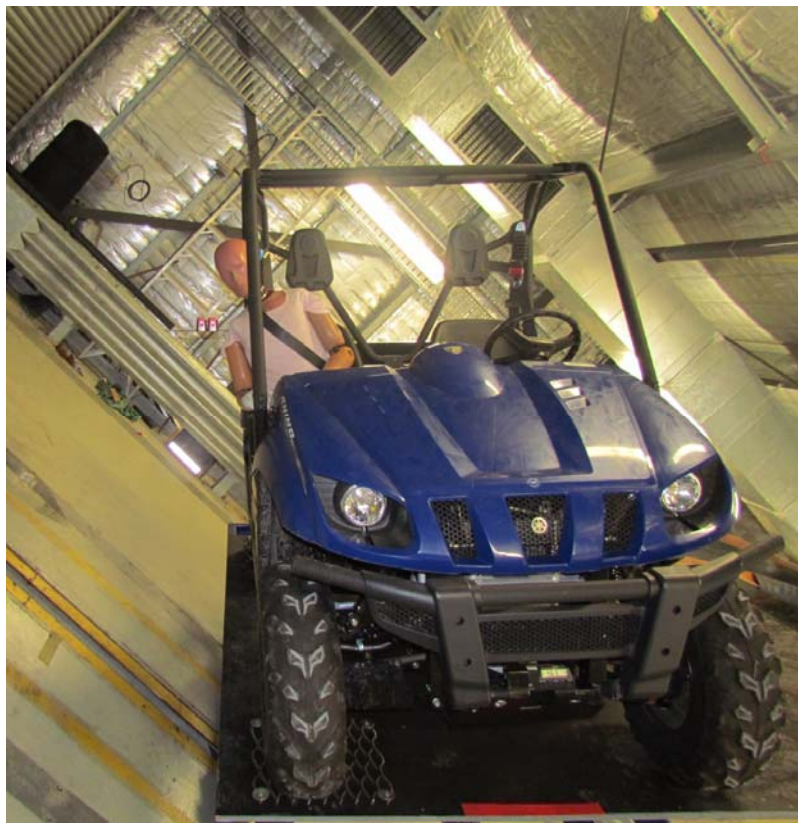
Side by Side Vehicle occupant retention – Test GI40064
