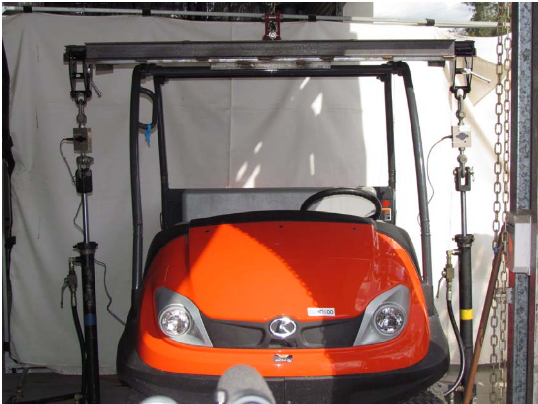
SSV ROPS test – Vertical test GI40100
