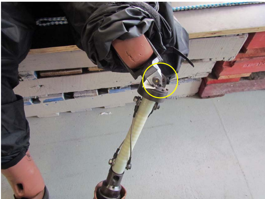
Vehicle and occupant rollover – Test latroll_01, damage to MATD left knee varus valgus shear pin
