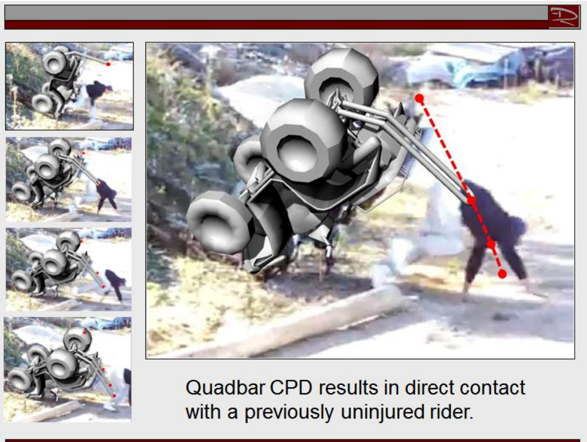
Figure 4: Van Ee et al. (2012) graphically present the hypothesis that a vehicle pitching forward over a rider could firstly obstruct the rider from potentially running out from under the Quad bike (left frame sequence) and secondly could potentially stab a person in the head, neck or back.
