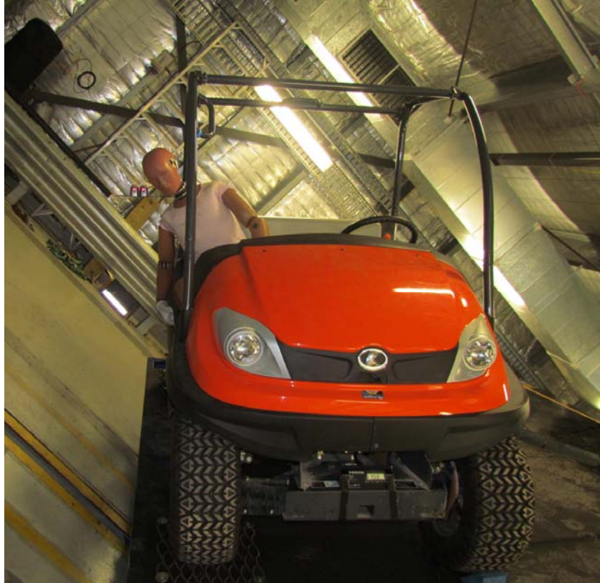
Side by Side Vehicle occupant retention – Test GI40057
