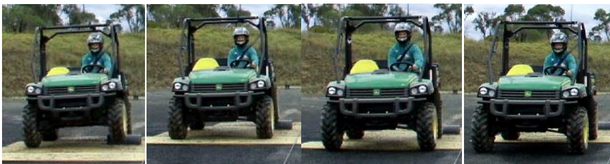
Figure 26: John Deere Gator passes over bump at 25 km/h with only slight vertical disturbance to driver or vehicle.
