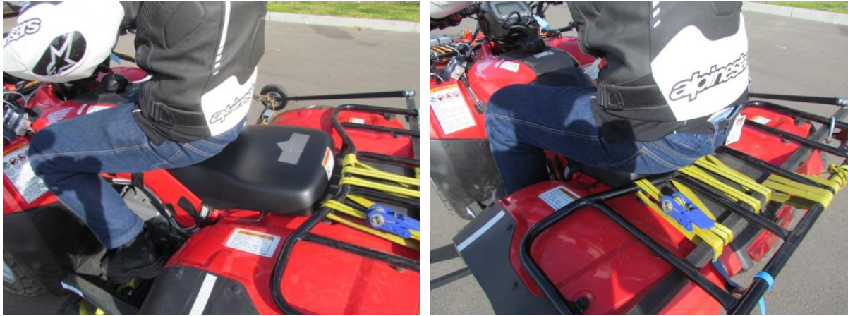
Figure 12: Showing riding position fully forward (left frame) and fully rearward (right frame).
