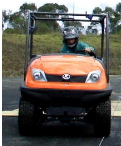
Figure 29: Vehicle ended up facing toward the camera, approximately 6 degrees of yaw.
