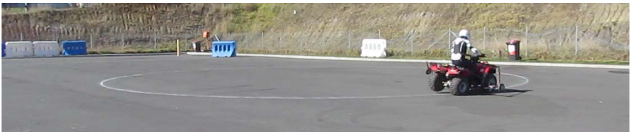
Typical quad bike Circular driving behaviour test (GI 30449) – rear wheel lifted
