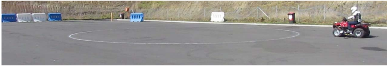
Typical quad bike Lateral transient response test (G130455)
