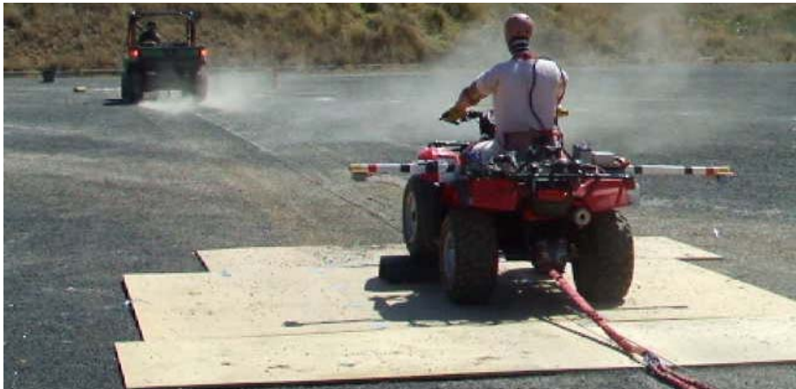
Typical quad bike Bump obstacle perturbation test (G130917)
