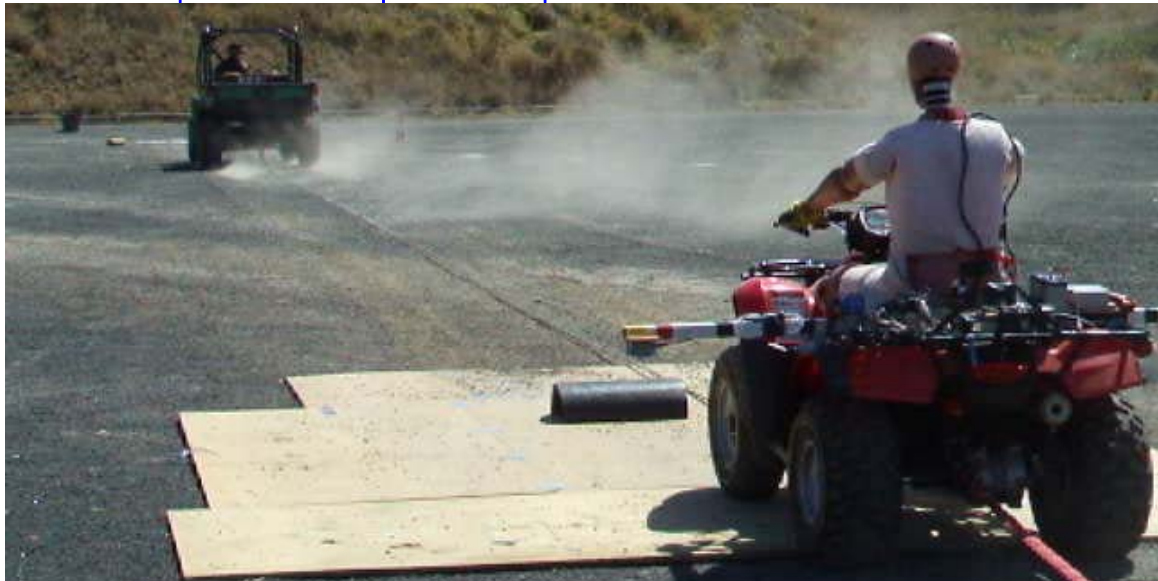
Typical quad bike Bump obstacle perturbation test (G130917)
