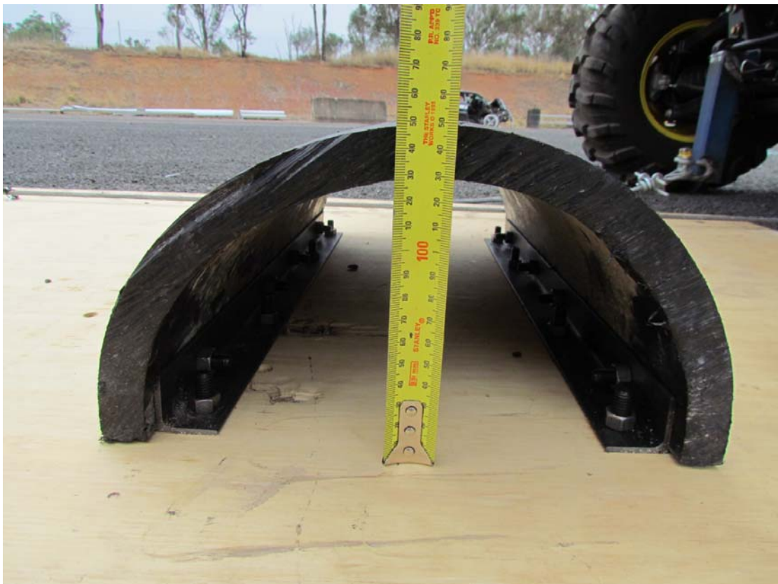
Bump obstacle (semi-circular, 150mm high)
