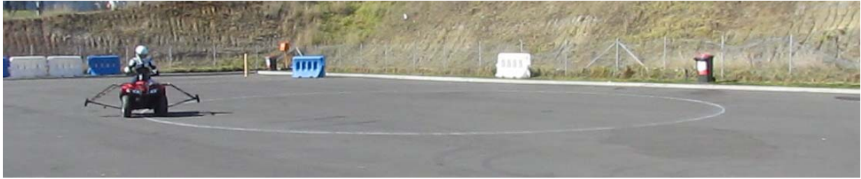
Typical quad bike Circular driving behaviour test (GI 30449)
