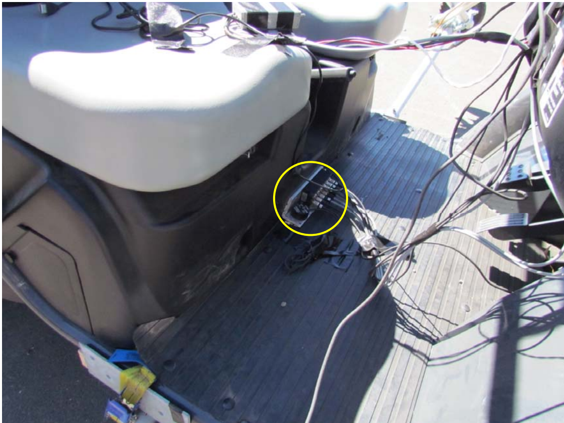
Data acquisition system, accelerometers and rate gyro installed close to COG (typical installation)
