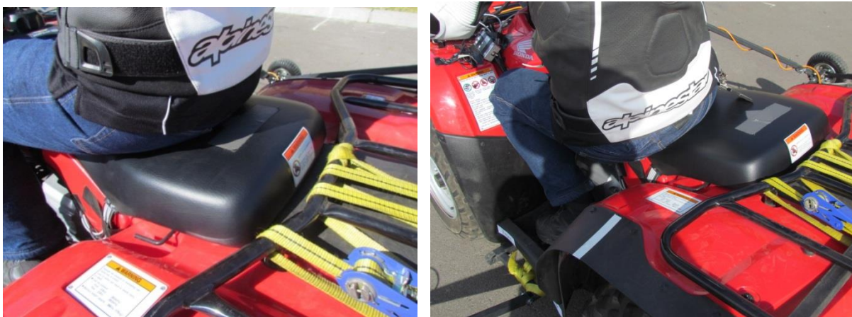
Figure 11: (left frame) Rider sitting at the seat reference point; (right frame) body shifted inward, forward and torso leaning into the turn. Rider weight is transferred forward and also to the inside footrest by this movement. Rollover resistance is thus improved by this.
