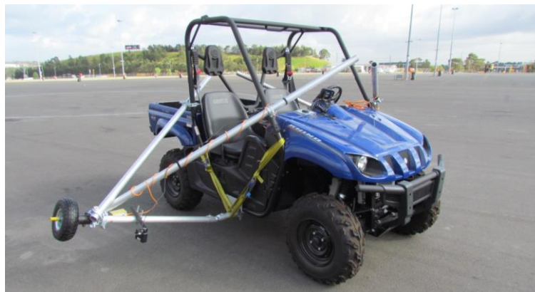
Figure 7: Steady state circle testing on asphalt and on grass. Top left: Rider on Quad bike following circle. Top right: Rider on Quad bike following grass circle at point of tilt. 2 nd row: Grass circle test site 3 rd row: Typical Quad bike circular driving behaviour test (G130449) – both wheels lifted. Bottom: Yamaha Rhino SSV with outrigger wheels.
