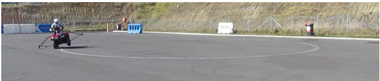
Typical quad bike Circular driving behaviour test (GI 30449) – both wheels lifted
