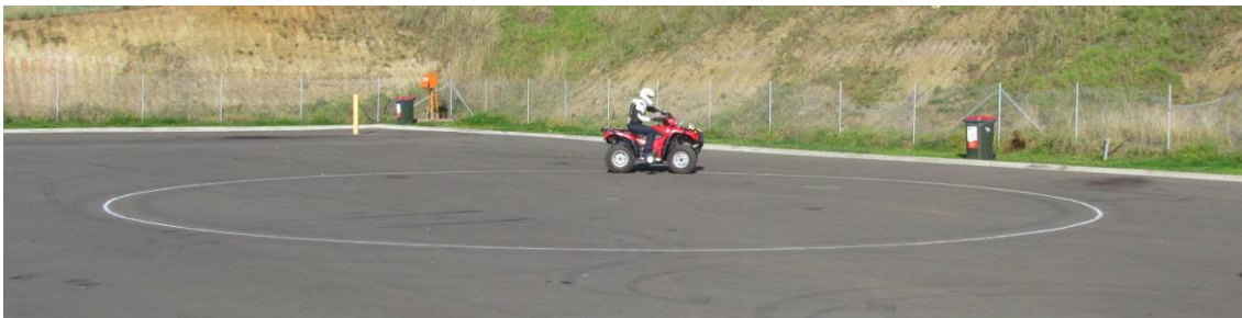
Figure 1 – steady state circular driving behaviour test in progress
