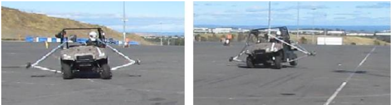
Figure 21: Honda Big Red MUV with open differential on left. Vehicle follows path of test circle easily and top speed is limited by inside rear wheel lift (spin-up). With locked differential on right, MUV oversteered throughout the test, ending up turning into the test circle, sliding sideways to the intended direction of travel and nearly tipped up onto the outrigger wheel.
