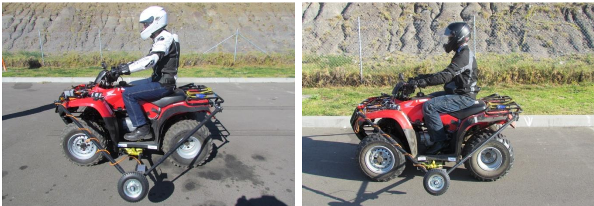
Figure 10: Different riders undertaking back to back testing. Results obtained (Attachment 1) show the vehicle characteristic is not rider dependant.
