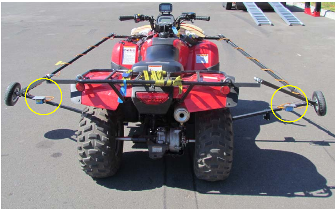
Distance measurement lasers (typical installation)
