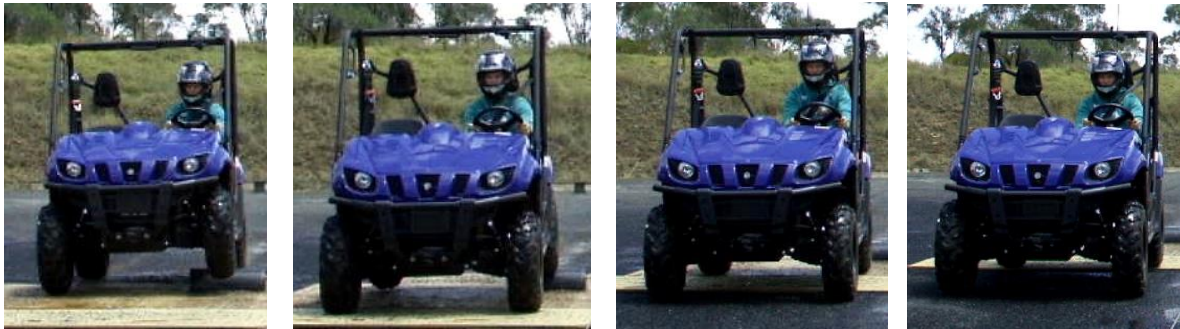
Figure 25: Yamaha Rhino passes over bump at 25 km/h with minimal disturbance to driver or vehicle.
