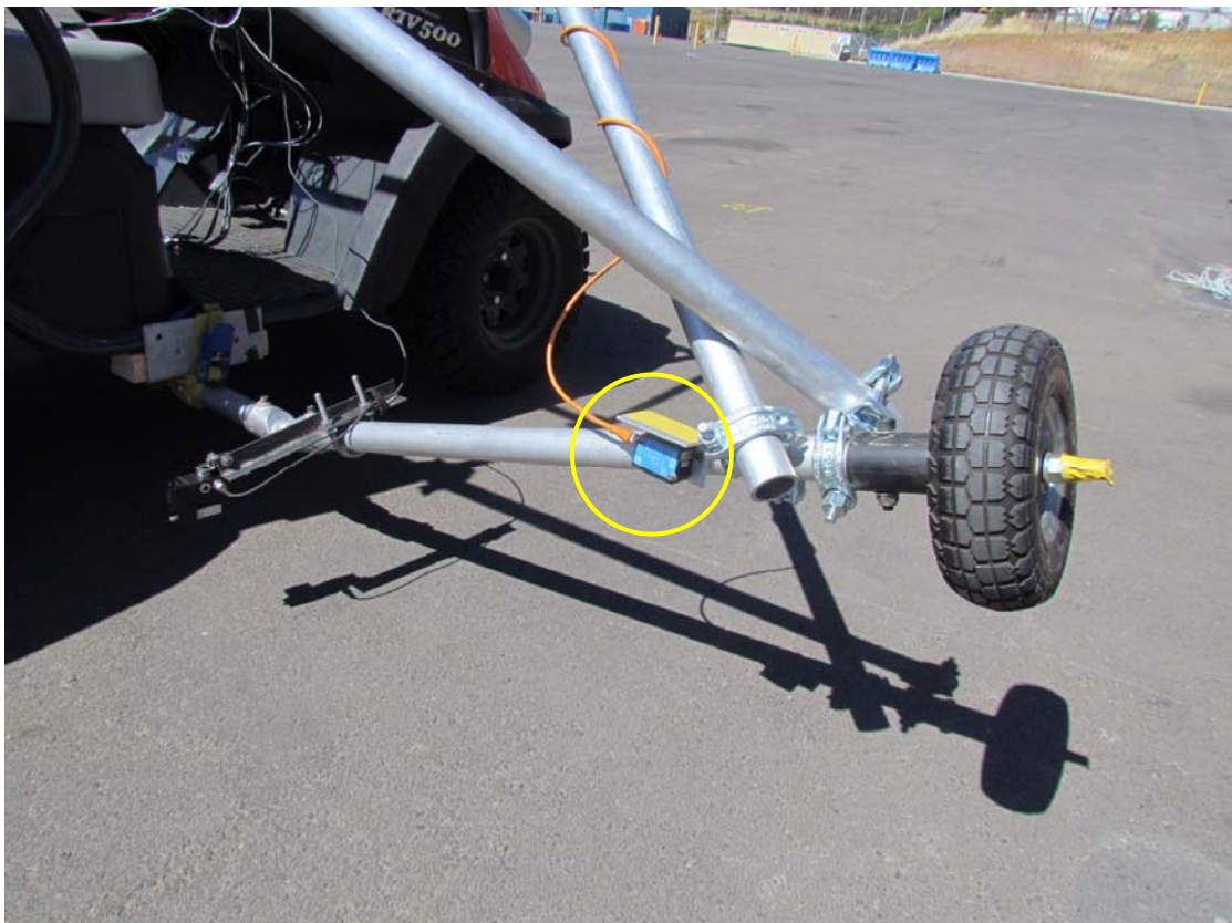
Distance measurement lasers (typical installation)
