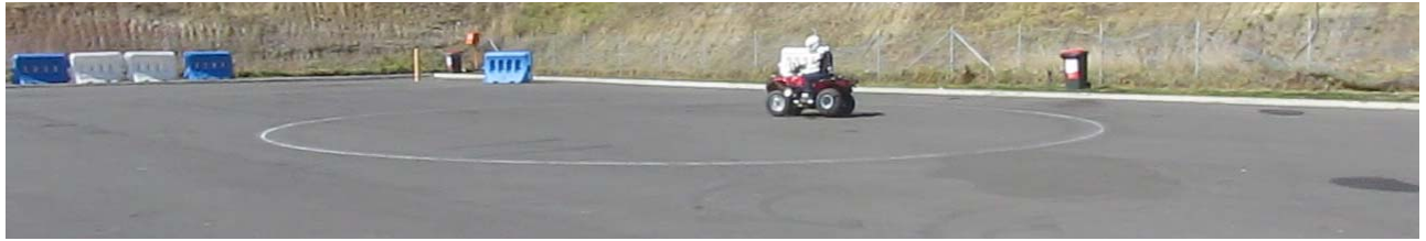
Typical quad bike Lateral transient response test (G130455)
