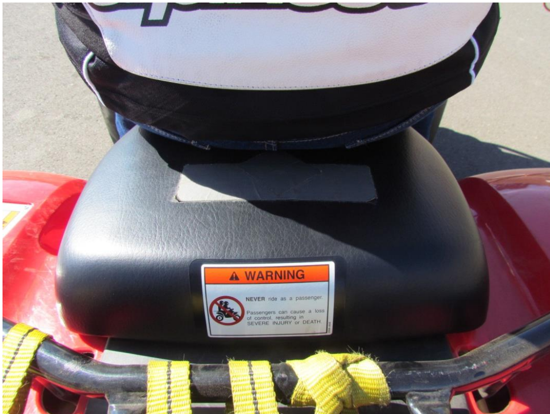
Figure 9: Use of the seat reference position to ensure the rider was sitting in the correct position on the saddle prior to each test run
