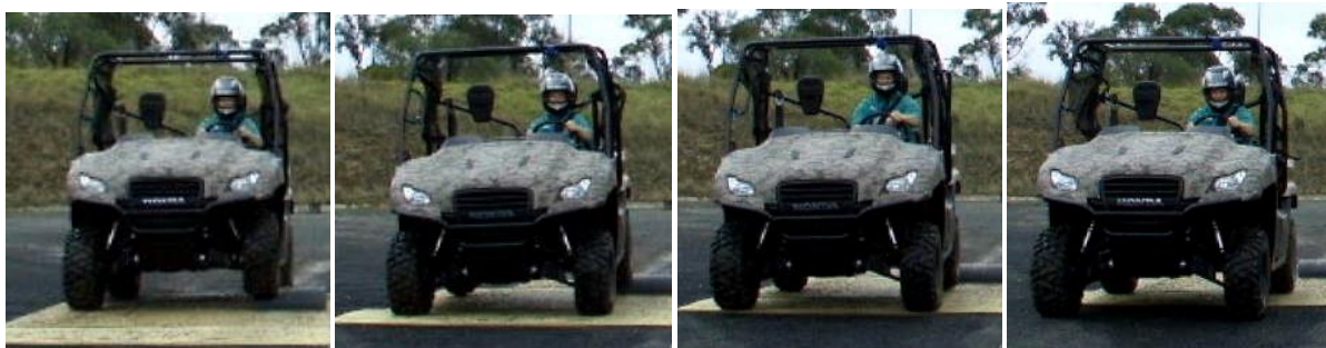
Figure 27: Honda Big Red MUV passes over bump at 25 km/h with only slight vertical disturbance to driver or vehicle.
