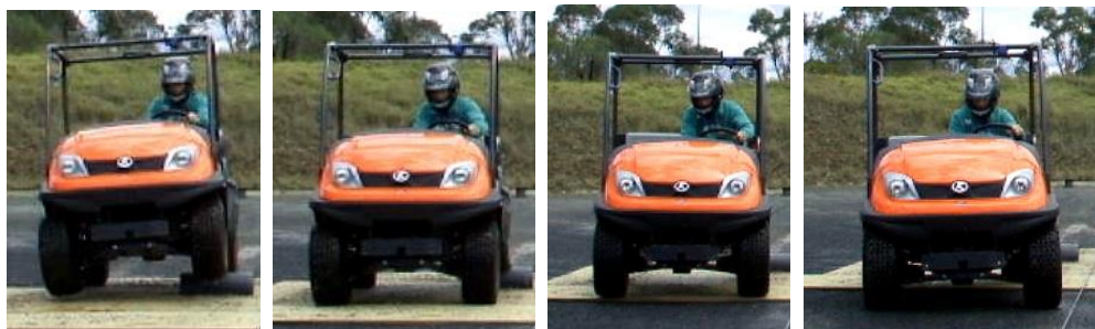
Figure 28: Kubota RTV 500 passes over bump at 25 km/h with minor visible vertical and lateral disturbance to vehicle and driver who holds on to the steering wheel.
