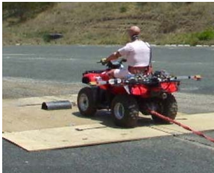
Figure 2 – bump obstacle perturbation test in progress
