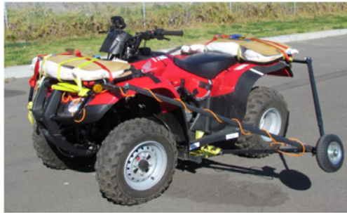
Front and Rear combined sandbag loads sandwiched by plywood
