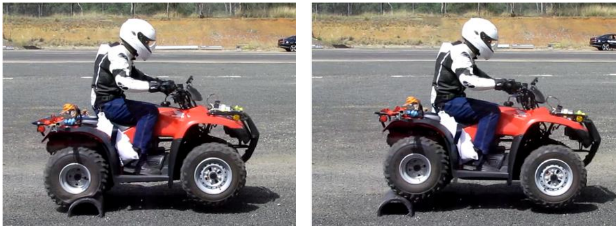
Figure 15: Negotiating a 100mm bump obstacle at 25 km/h (ballasted to 103 kg load). The low pressure tyre bottoms out, as has the suspension travel, forcing the Quad bike and rider to rise up over the obstacle. This creates vertical and lateral accelerations for the rider that can be measured by the test protocol.
