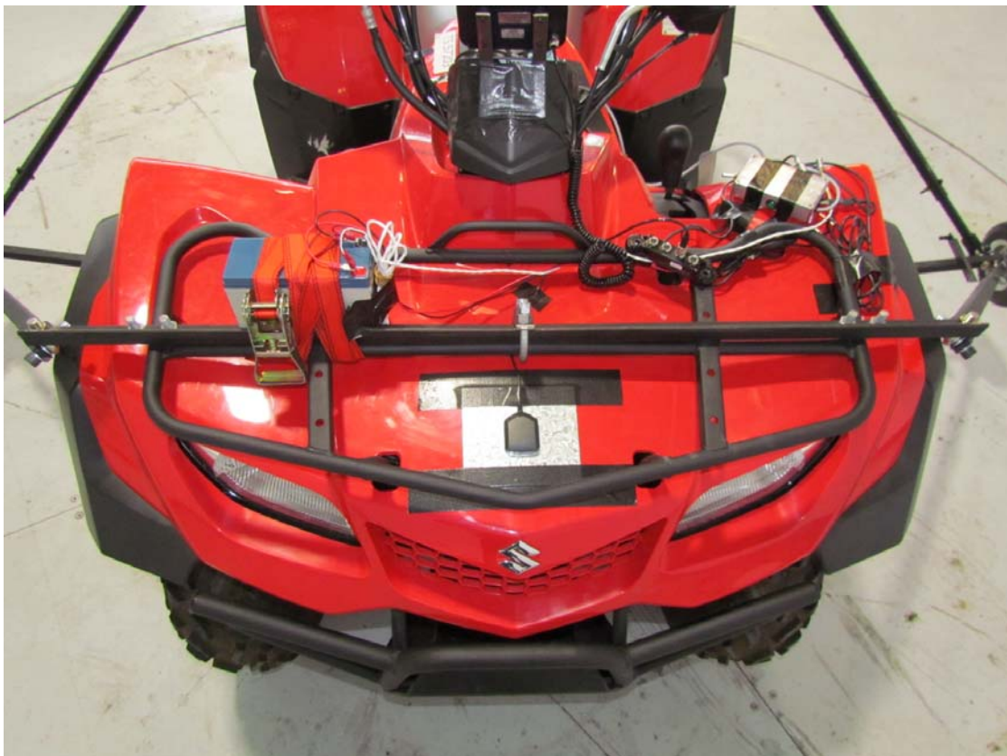
GPS antennae, battery and ancillary equipment (typical installation)
