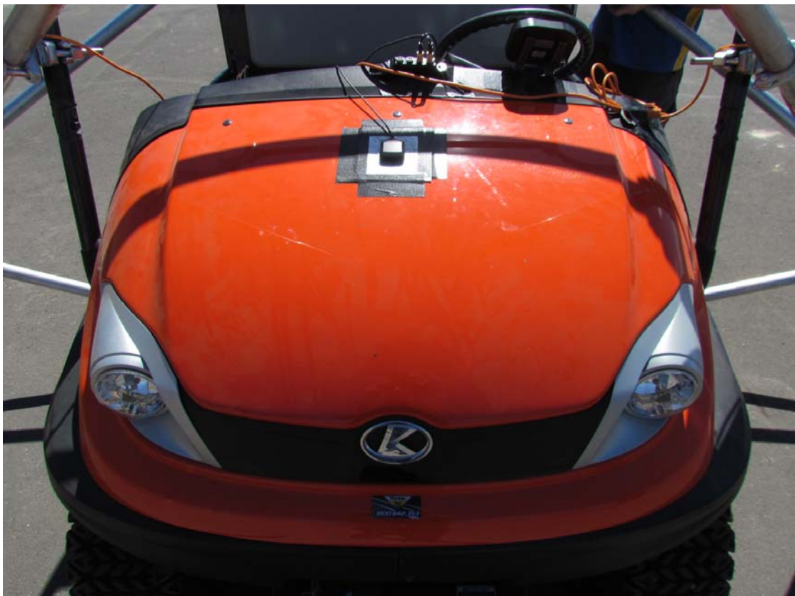
GPS antennae and ancillary equipment (typical installation)
