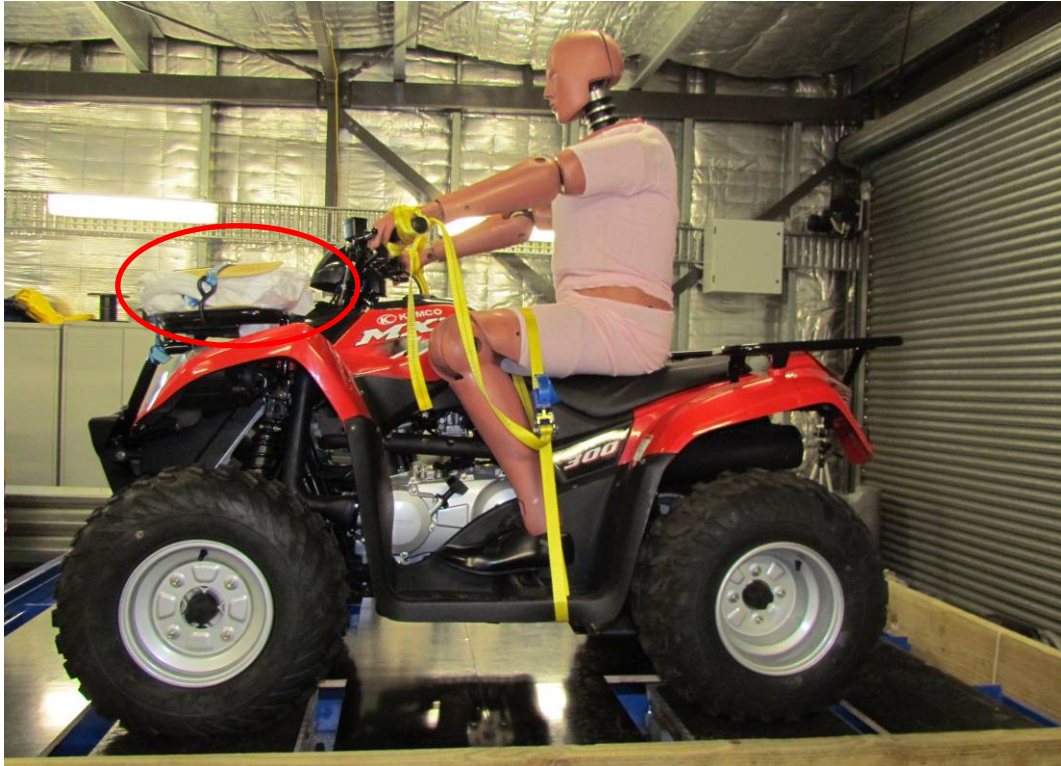
Typical ATV setup - with ATD and front load (GI 30005)
