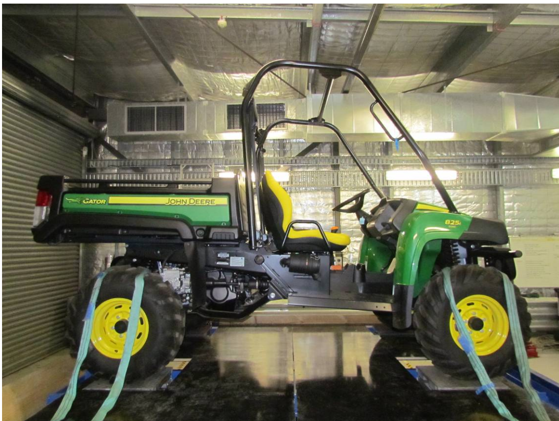
Typical SSV set up for lateral roll test (G130316)
