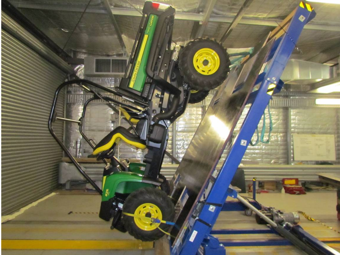
Typical SSV forward pitch test, vehicle liftoff (G1 30319)
