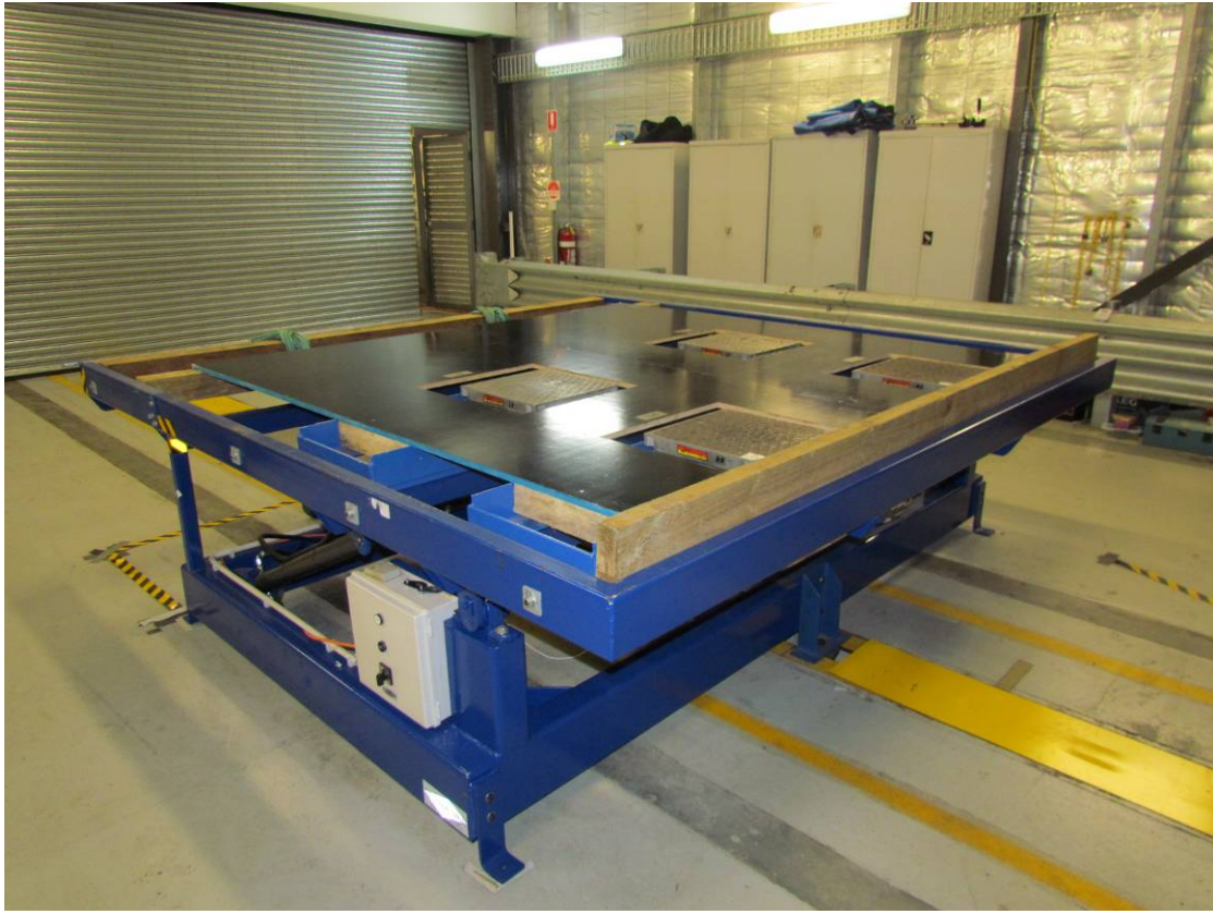
Tilt table (lowered, horizontal position)
