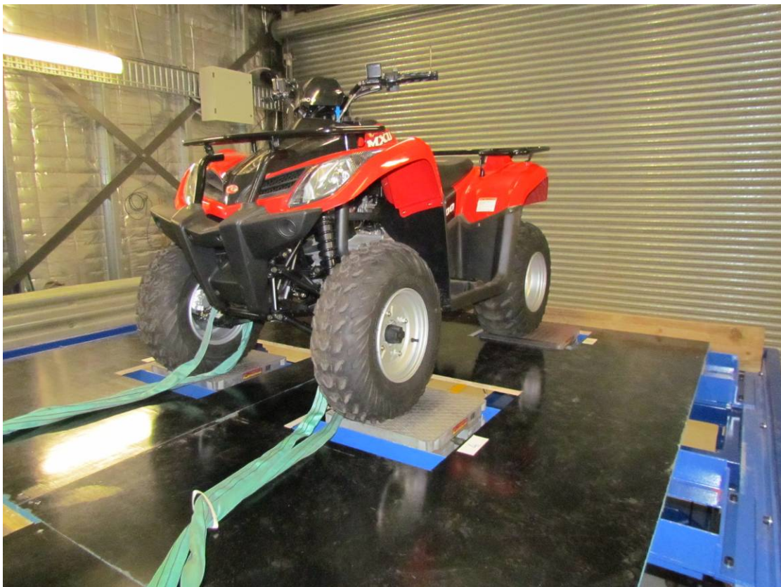
Typical ATV set up for rearward pitch test (GI30165)
