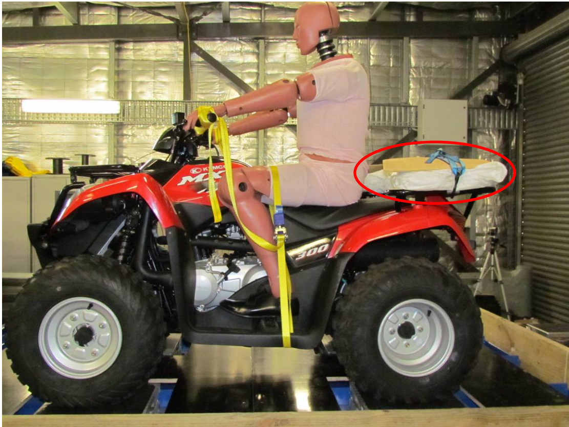
Typical ATV setup - with ATD and rear load (GI 30009)
