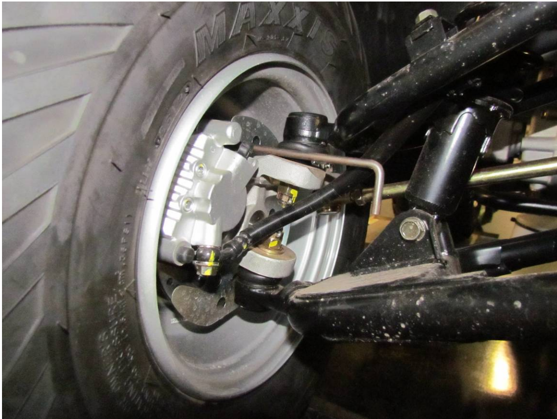
Typical locking of ATV front brakes for forward pitch test (GI30156)
