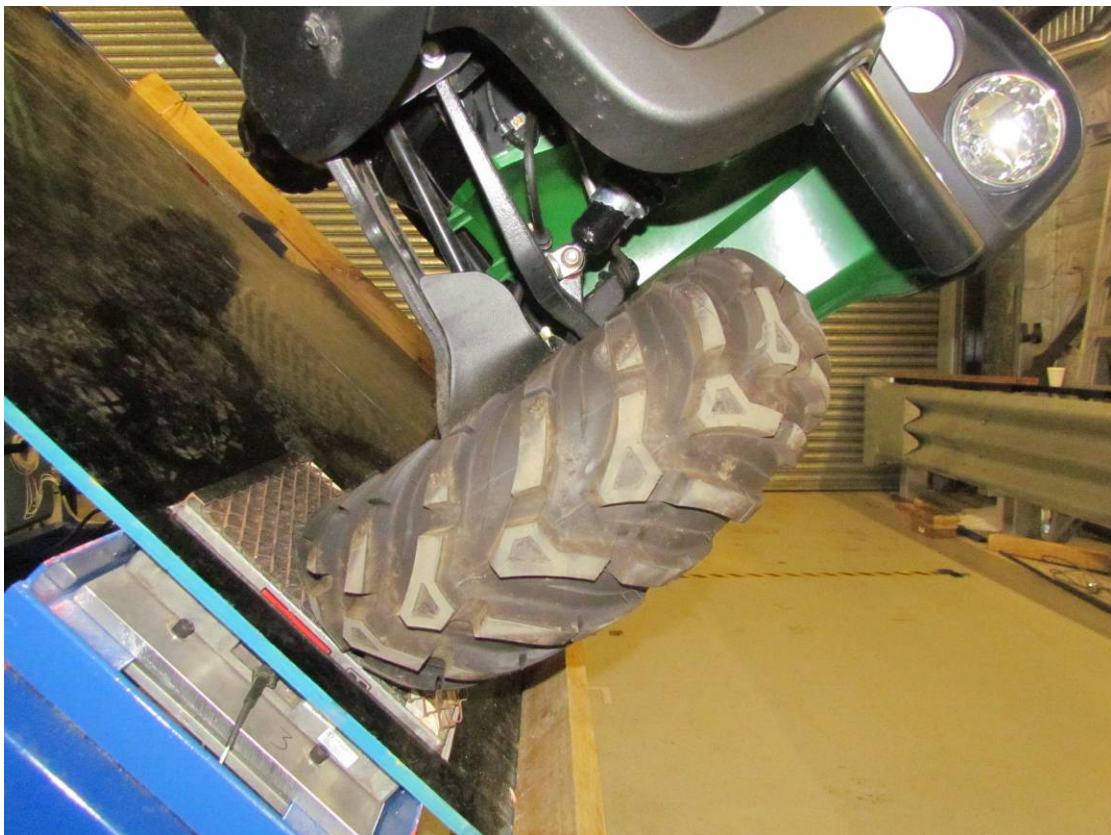
Typical ATV lateral roll test, tyre squirm at vehicle liftoff (G130316)
