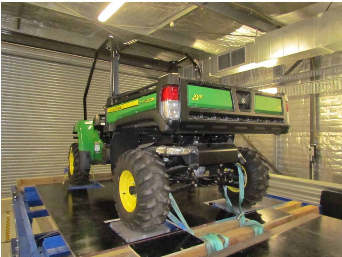
Typical SSV set up for forward pitch test (GI 30319)
