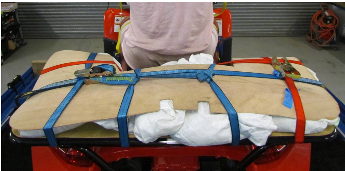
Typical ATV setup - rear load fastening, load distributed on cargo rack
