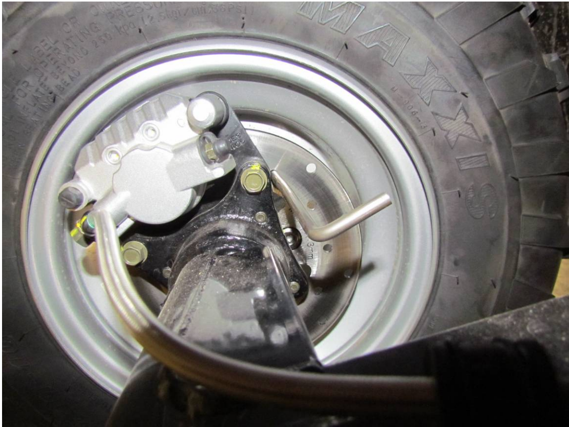
Typical locking of ATV rear brakes for rearward pitch test (G130165)
