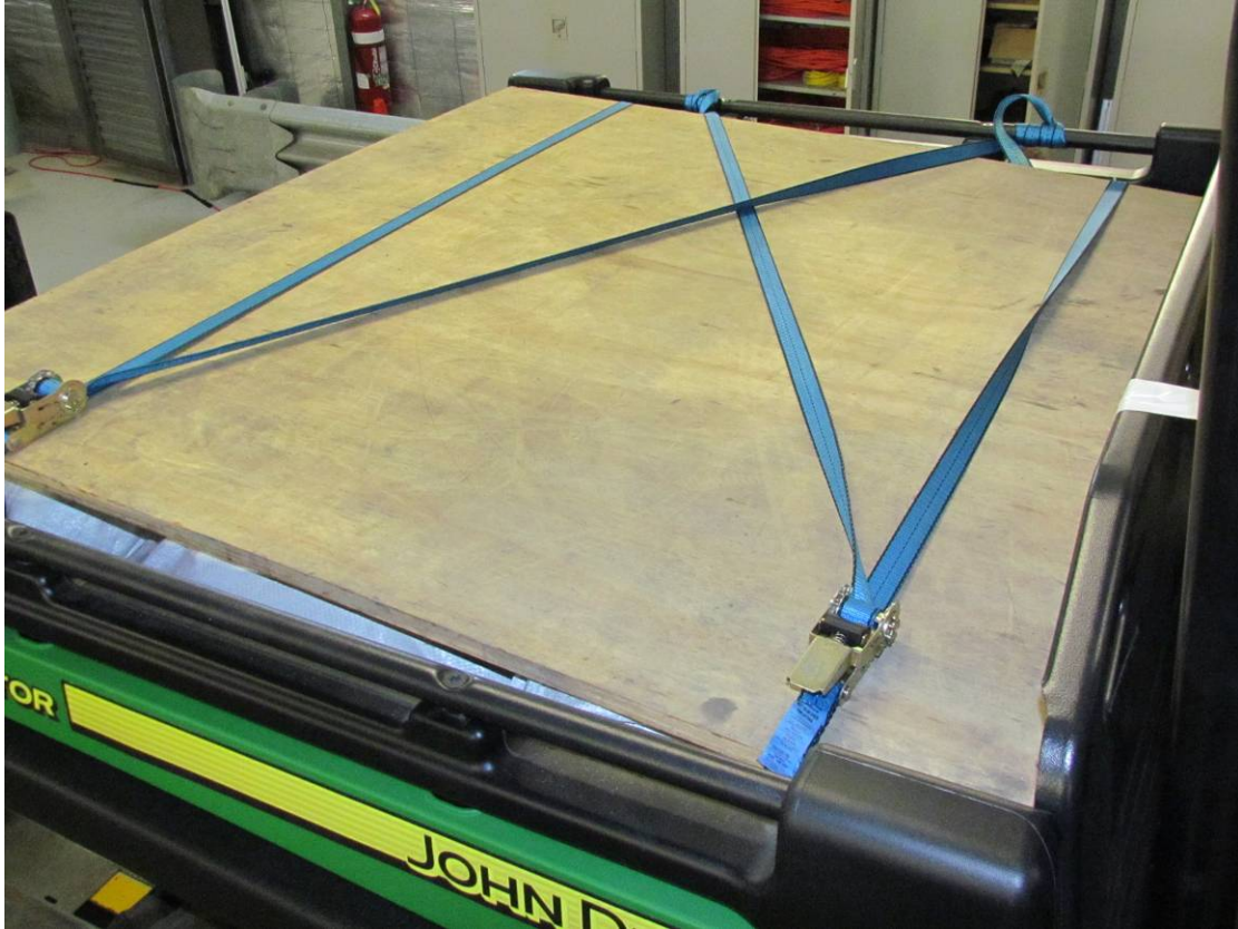
Typical SSV setup - rear load fastening, load distributed in utility tray
