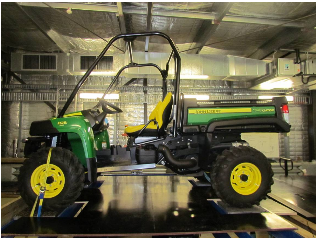
Typical SSV setup - no load (GI30319)
