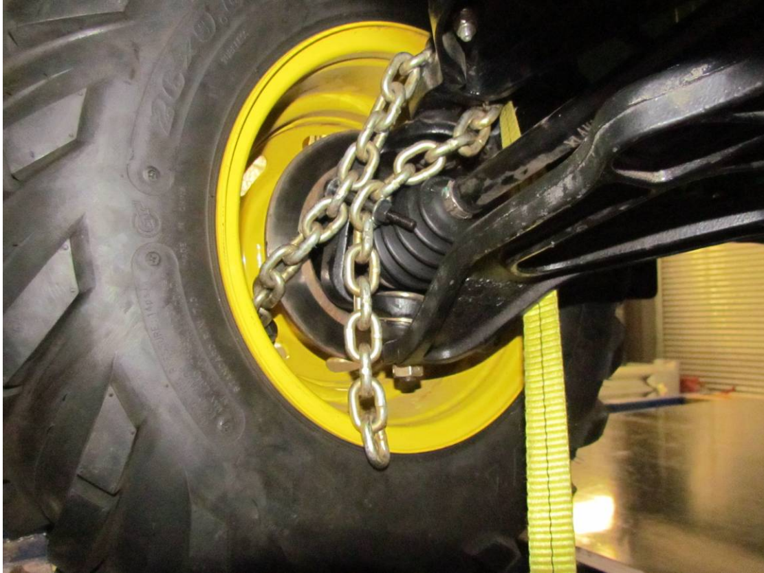
Typical locking of SSV front wheels for forward pitch test (G130319)
