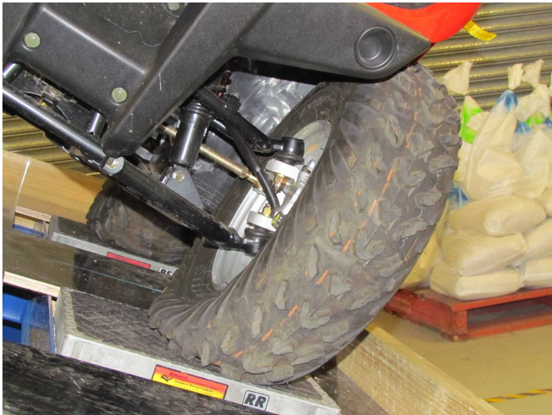
Typical ATV lateral roll test, tyre squirm at vehicle liftoff (G130005)
