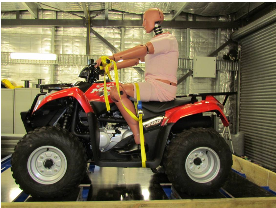
Typical ATV setup – with Hybrid III 95%ile ATD (G130003)
