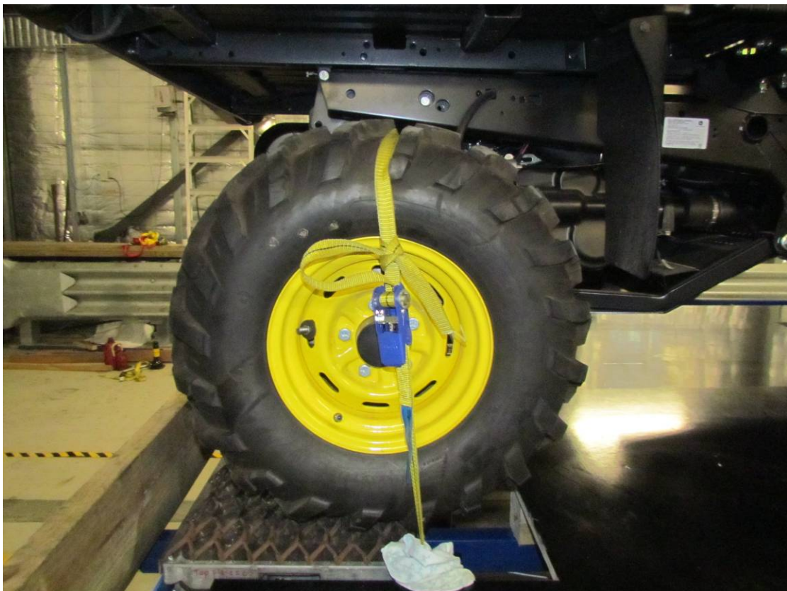
Typical vertical strapping of SSV rear wheels to load cell for rearward pitch test (GI 30324)
