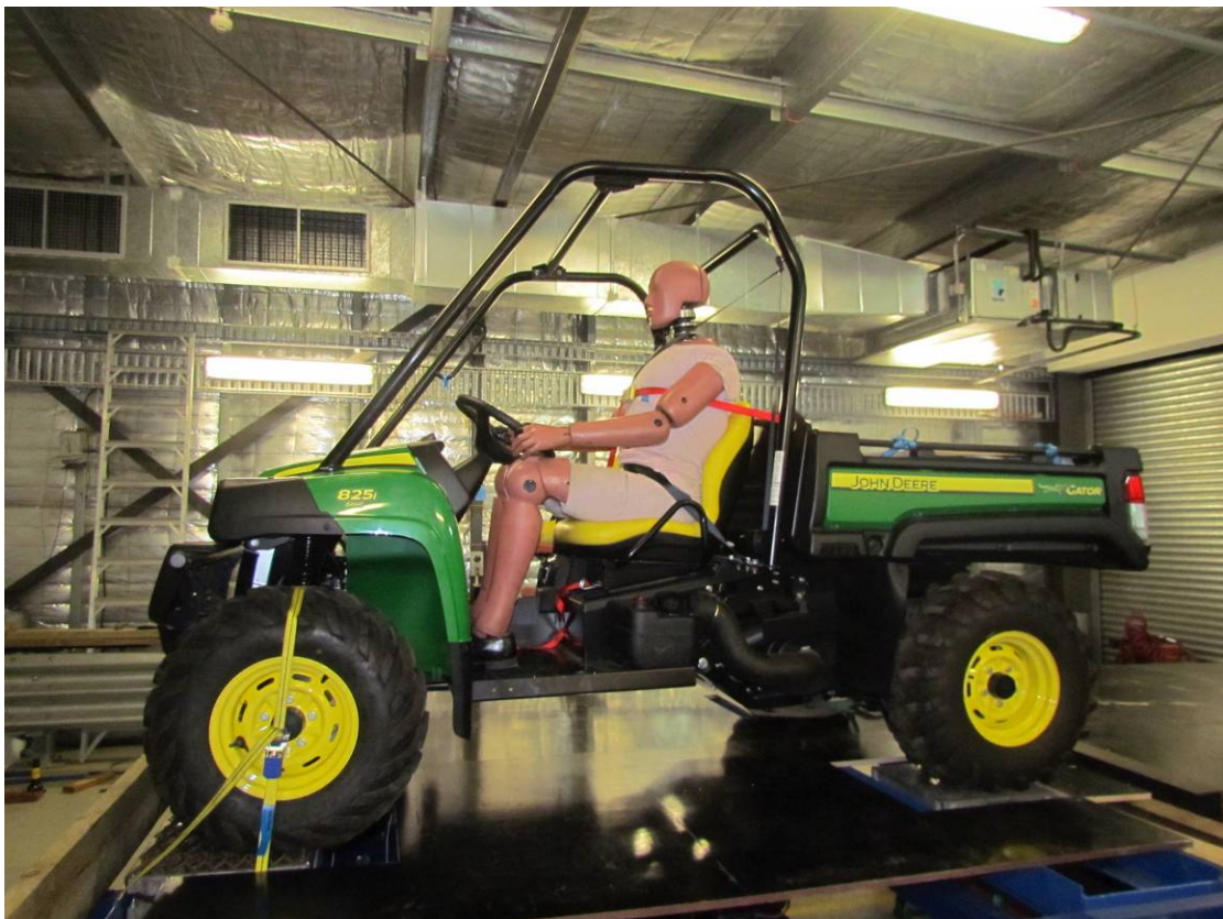
Typical ATV setup - with ATD and rear load (GI 30321)
