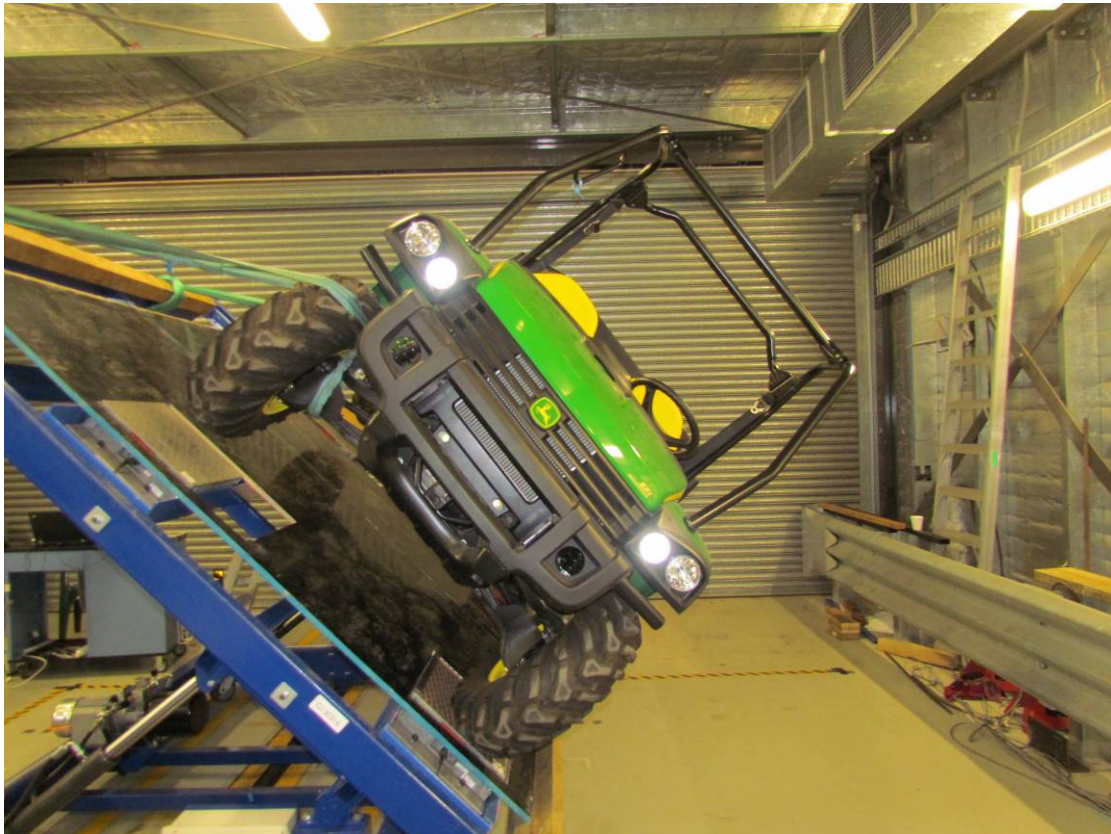
Typical SSV lateral roll test, vehicle liftoff (G130316)
