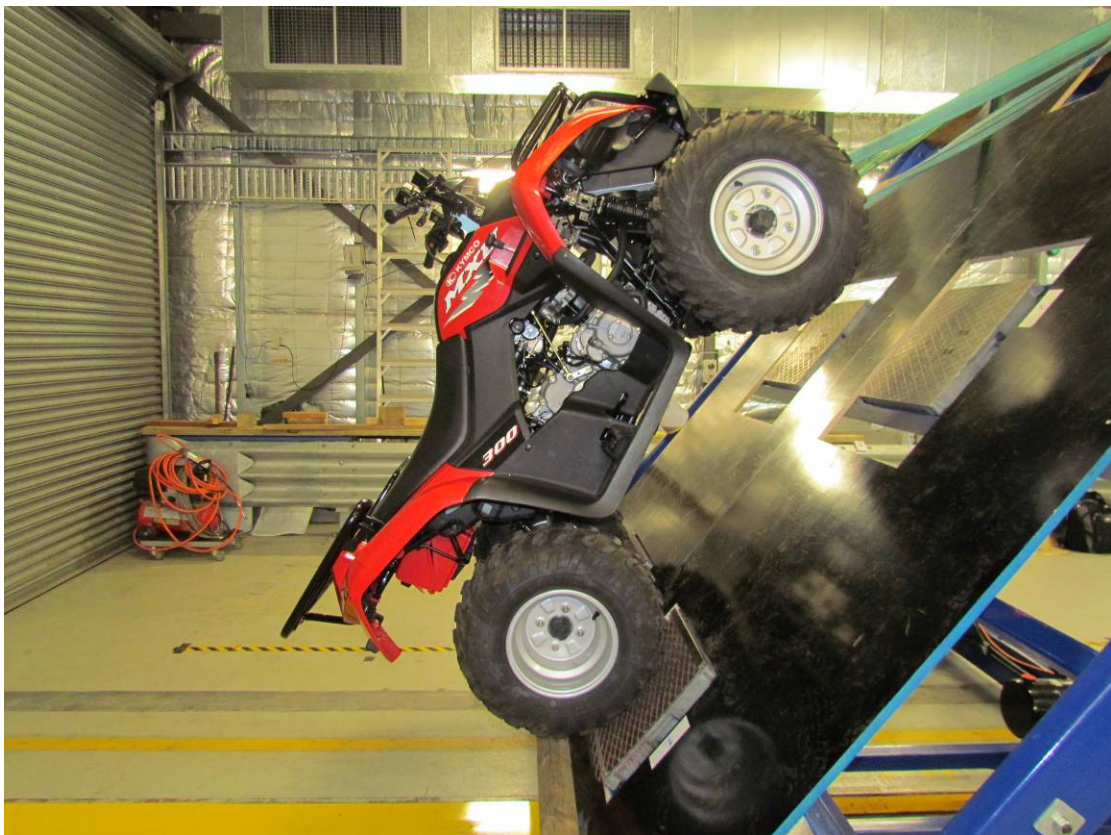
Typical ATV rearward pitch test, vehicle liftoff (G130165)
