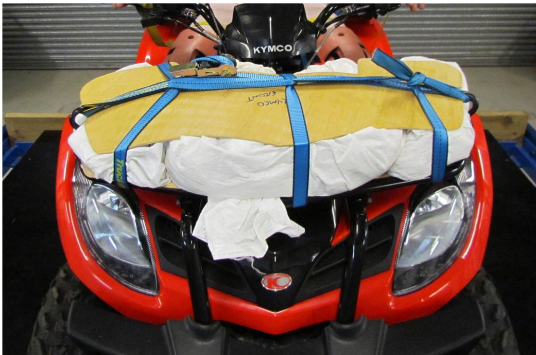
Typical ATV setup - front load fastening, load distributed on cargo rack
