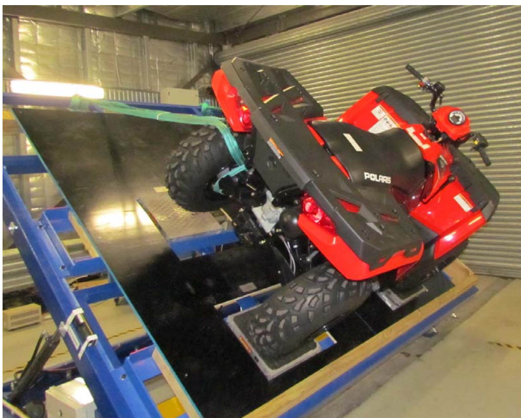
Figure 1: Single axis tilt table with quad bike
