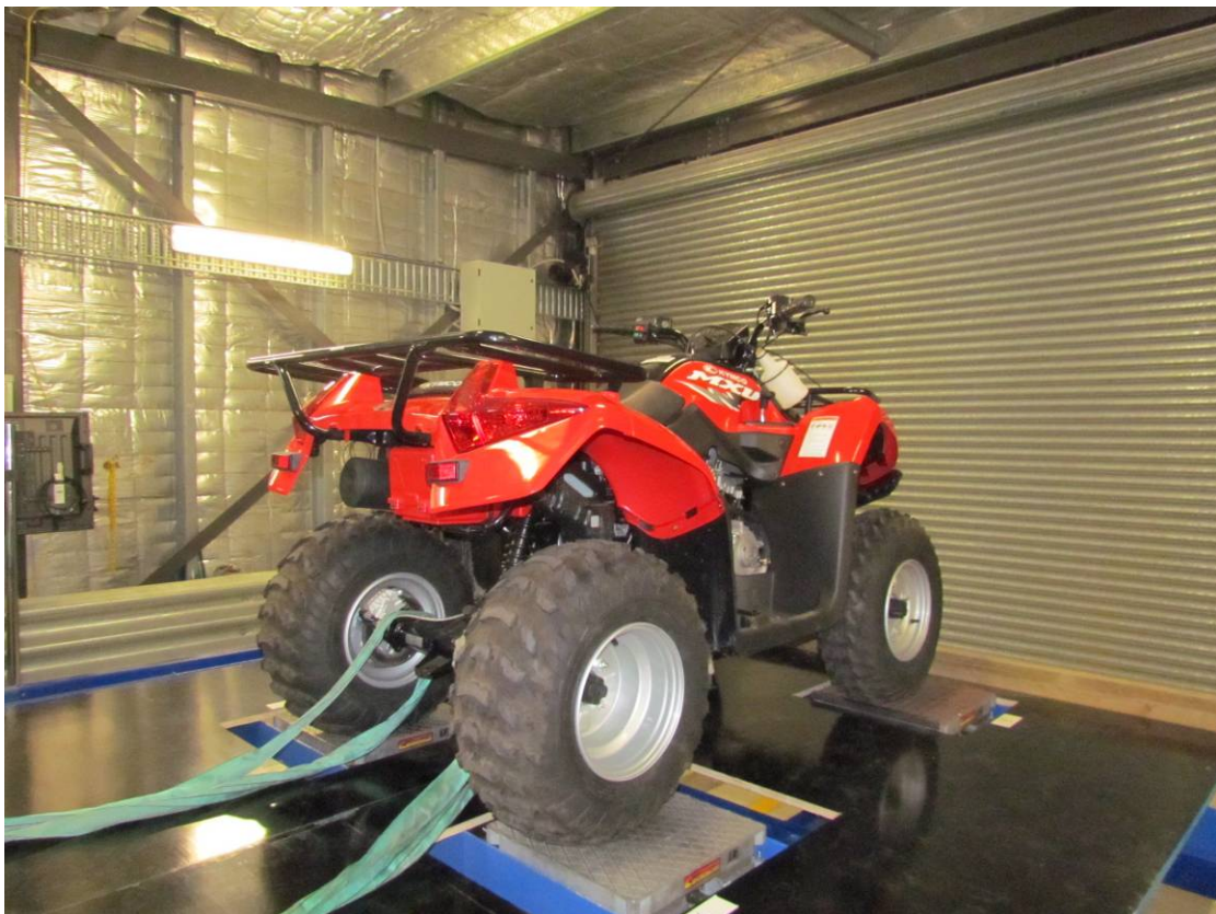
Typical ATV set up for forward pitch test (G130156)
