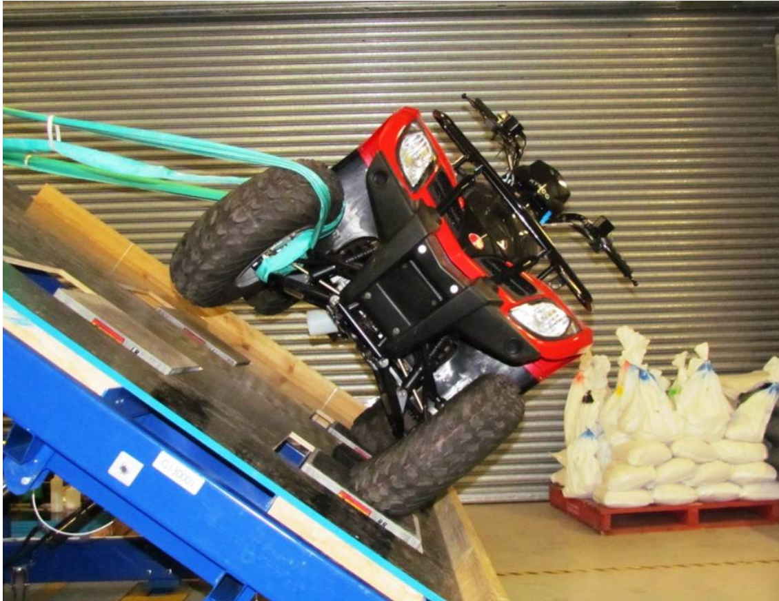
Typical ATV lateral roll test, vehicle liftoff (G130001)
