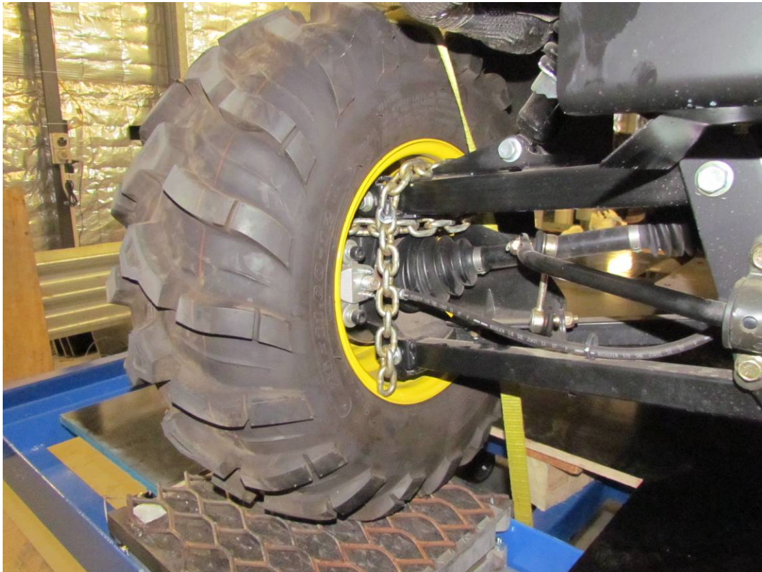
Typical locking of SSV rear wheels for rearward pitch test (GI 30324)
