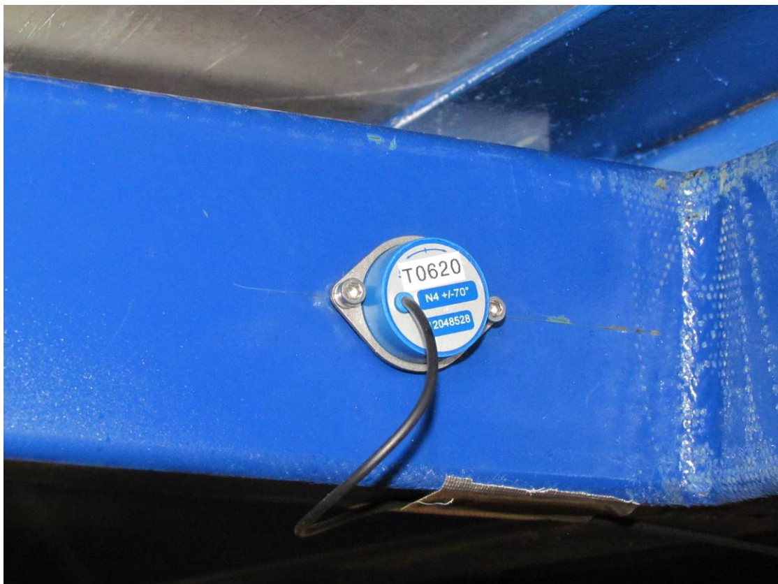
Tilt table tilt sensor, mounted to upper table frame
