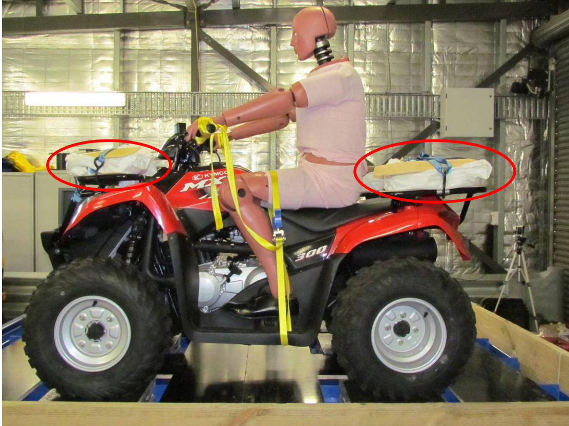
Typical ATV setup - with ATD, front load and rear load (GI 30007)
