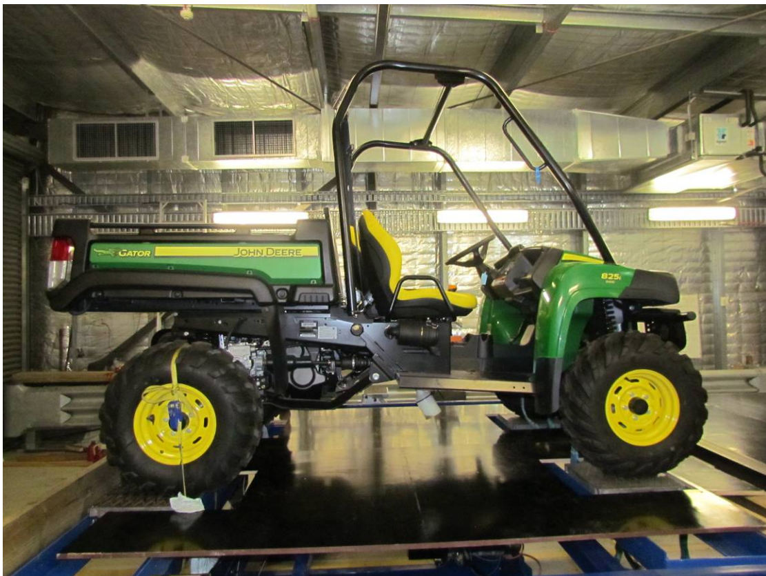
Typical SSV set up for rearward pitch test (G1 30324)
