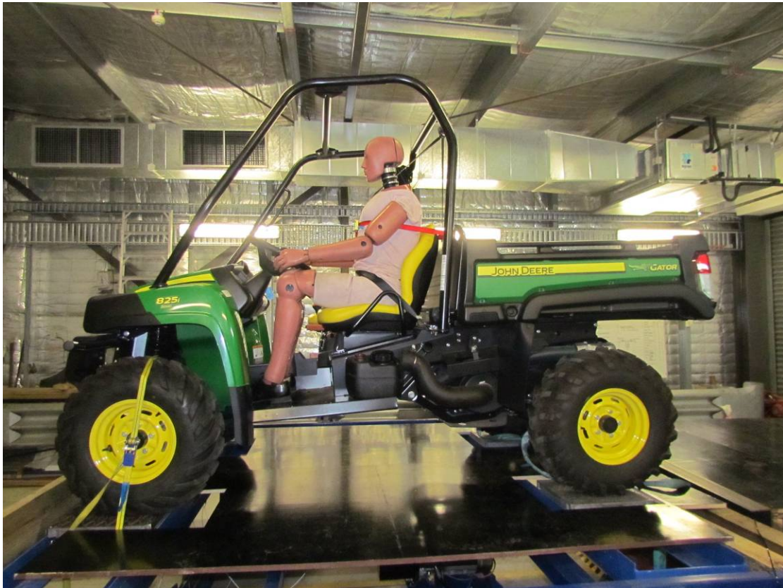
Typical SSV setup - with Hybrid III 95%ile ATD (GI 30320)
