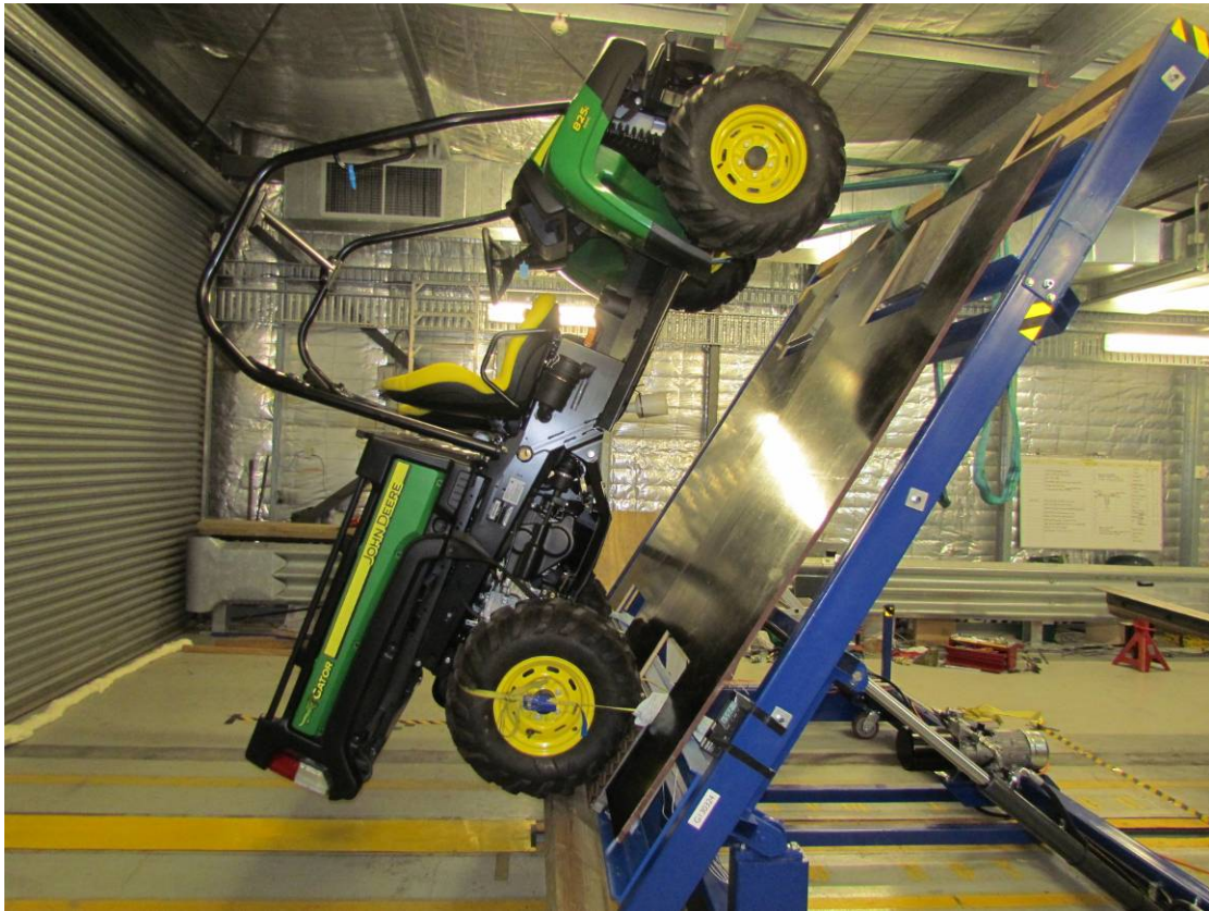
Typical SSV rearward pitch test, vehicle liftoff (GI 30324)
