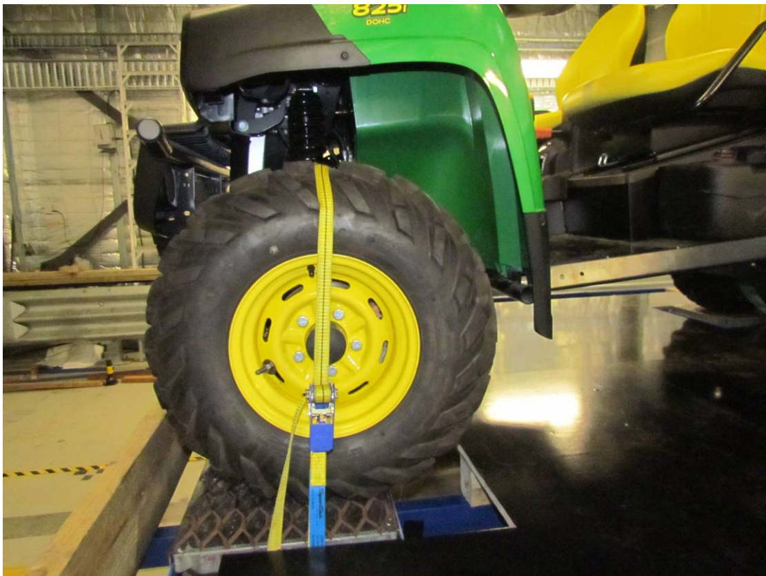
Typical vertical strapping of SSV front wheels to load cell for forward pitch test (G130319)
