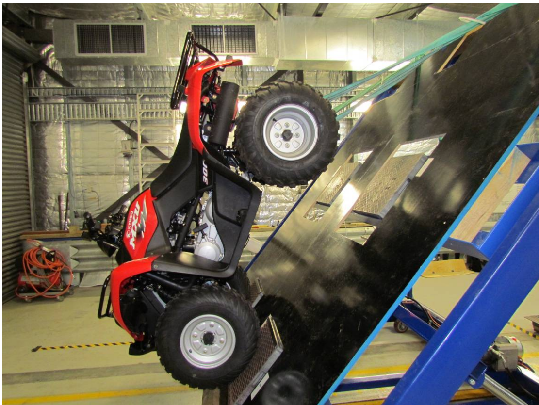
Typical ATV forward pitch test, vehicle liftoff (GI30156)
