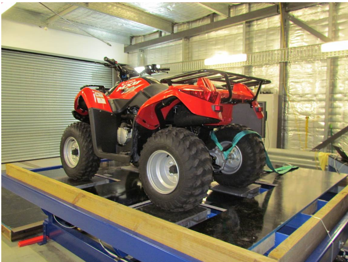
Typical ATV set up for lateral roll test (GI 30001)
