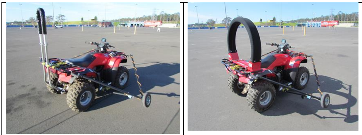
Figure 9: Quad bike vehicle setup – with OPDs (Quadbar and Lifeguard).
