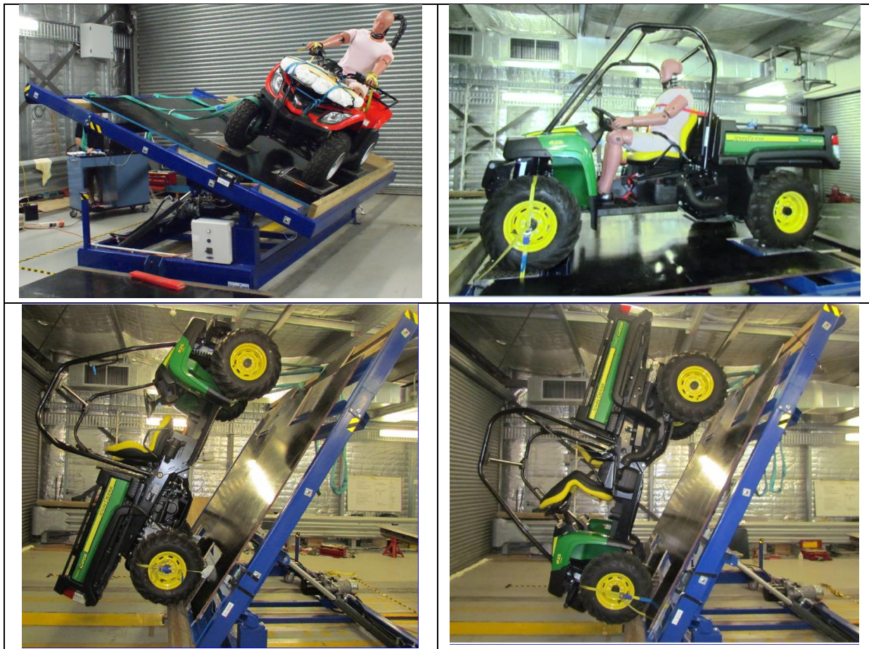
Figure 4: Photographs from the tilt table tests, showing Quad bike with ATD and OPD for a lateral roll tests, and the John Deere SSV for lateral roll, rear and forward pitch tests.
