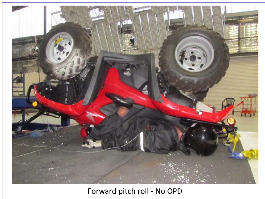
Figure 14: Examples of Quad bike lateral rollover and forward pitch tests with and without OPDs. For more details see 'Part 3: Rollover Crashworthiness Test Results' report.
