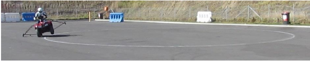
Figure 7: Typical quad circular driving behaviour test (G130449) – both wheels lifted.
