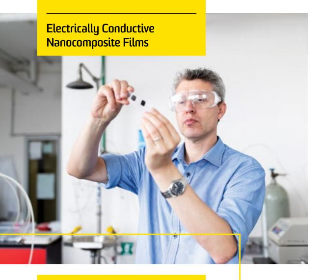
Synthesis of polymer nanoparticles with graphene oxide sheets via mini-emulsion polymerisation enabling electrically conductive films using an ambient temperature process. These films exhibit high electrical conductivity with a wide range of applications as conductive coatings.
